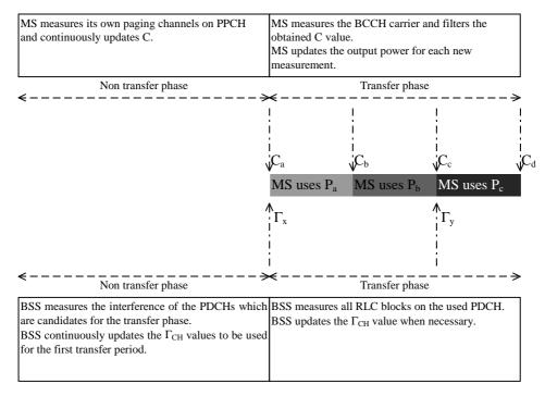
Figure B.1: Traffic example of uplink power control
