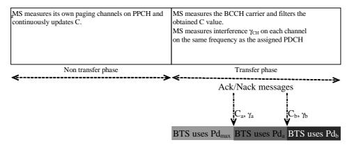
Figure B.2: Traffic example of downlink power control
