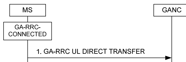
Figure 8a.2.3.1 Uplink direct transfer, normal flow
