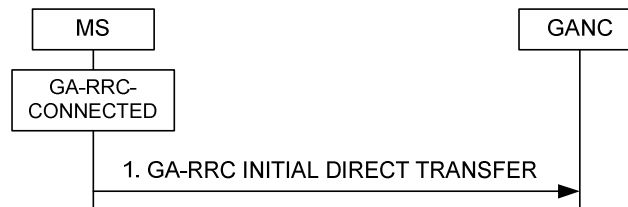
Figure 8a.2.1.1 Initial direct transfer, normal flow
