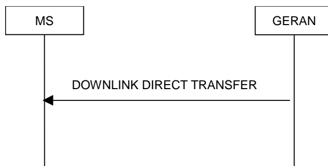
Figure 7.17.2.1: Downlink Direct transfer, normal flow
