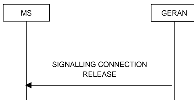
Figure 7.15.1.1.1: Signalling Connection Release procedure, normal case
