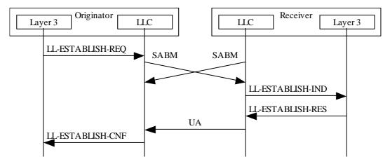
Figure 19: Collision between LLE-initiated and layer 3-initiated ABM establishment procedure
