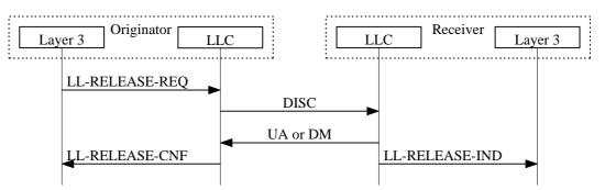
Figure 16: ABM release procedure
