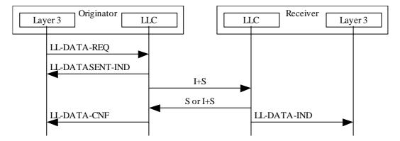
Figure 20: Transmitting and receiving I frames
