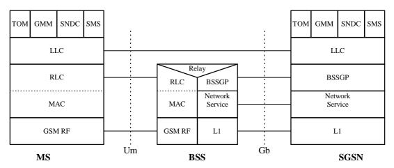
Figure 1: Protocol layering in GPRS
