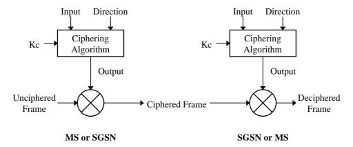
Figure A.1: GPRS ciphering environment
