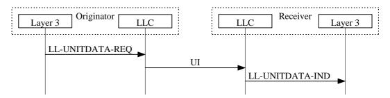
Figure 13: Unacknowledged information transmission
