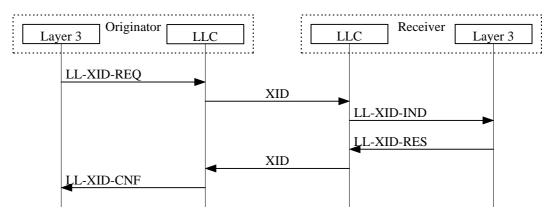
Figure 18: Layer 3 XID negotiation procedure
