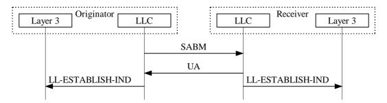
Figure 21: LLC-initiated ABM re-establishment procedure
