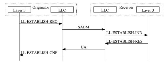
Figure 14: Layer 3-initiated ABM establishment procedure
