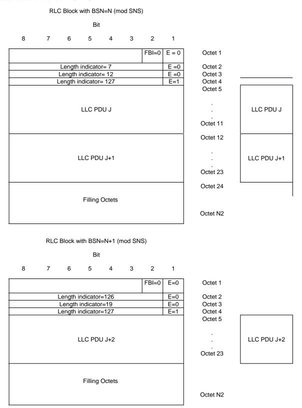
Figure B.11: Example for the case when the LLC PDU J+1 ends in the previous RLC data block and the start of the next LLC PDU J+2 is in the next RLC data block which is indicated using LI=126 as the first LI in that RLC data block.
