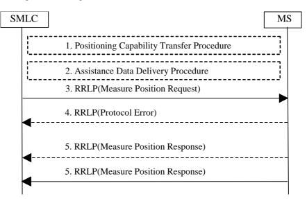
Figure 2.1: Position Measurement procedure
