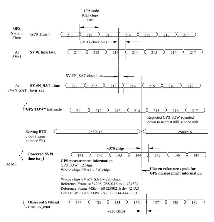
Figure A.1. Exemplary definitions of GPS measurement information fields.
