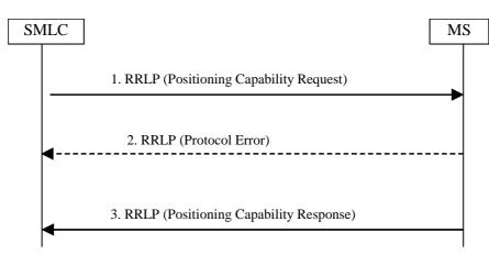
Figure 2.3: Positioning Capability Transfer procedure
