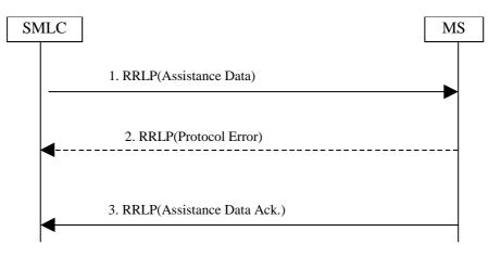
Figure 2.2: Assistance Data Delivery procedure
