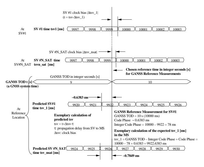
Figure A.4a. Exemplary calculations of some GANSS Reference Measurement fields with respect to GANSS TOD.
