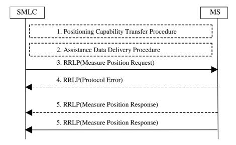
Figure 2.1: Position Measurement procedure
