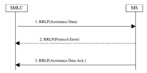
Figure 2.2: Assistance Data Delivery procedure
