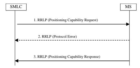
Figure 2.3: Positioning Capability Transfer procedure
