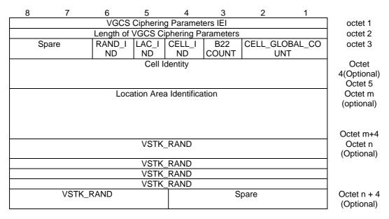
Figure 10.5.2.42b.1: VGCS Ciphering Parameters Information Element
