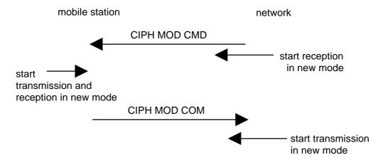
Figure 3.4.7.2.1: Ciphering mode setting sequence
