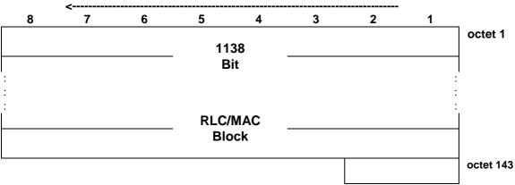
The numbering convention specified in GSM 44.060 applies. NOTE:
