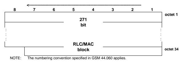
Figure 7.6: PDTCH block type 2 (CS-2) format
