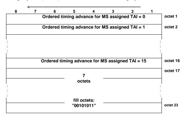
Figure 7.10: PTCCH downlink block format
