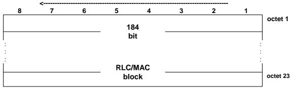
NOTE: The numbering convention specified in GSM 44.060 applies.
