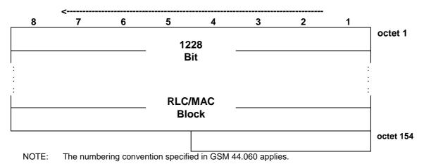
Figure 7.6.13.2: PDTCH block type 13 (MCS-9) downlink format
