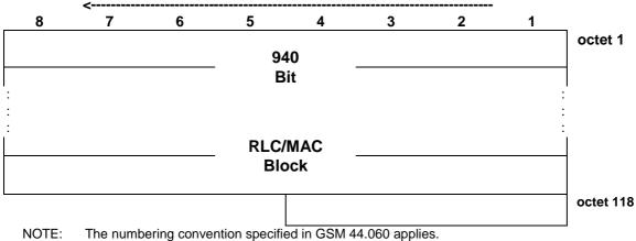
Figure 7.6.11.2: PDTCH block type 11 (MCS-7) downlink format
