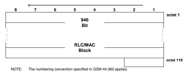
Figure 7.6.11.1: PDTCH block type 11(MCS-7) uplink format
