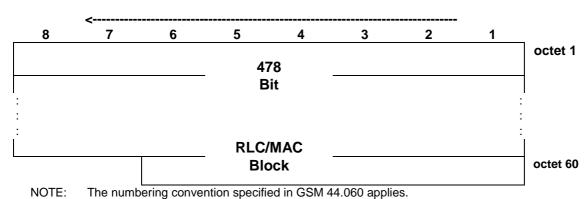
Figure 7.6.9.2: PDTCH block type 9 (MCS-5) downlink format
