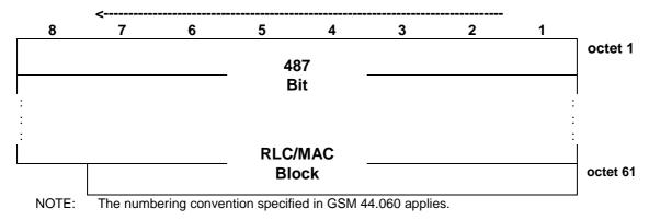
Figure 7.6.9.1: PDTCH block type 9 (MCS-5) uplink format
