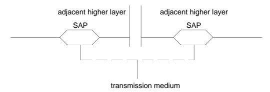
Figure 3.1: Service Access Point principle
