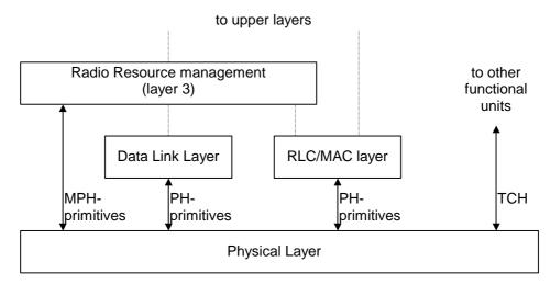
Figure 2.1: Interfaces with the Physical Layer
