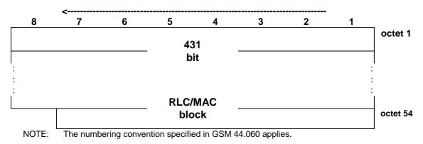
Figure 7.6.4: PDTCH block type 4 (CS-4) format
