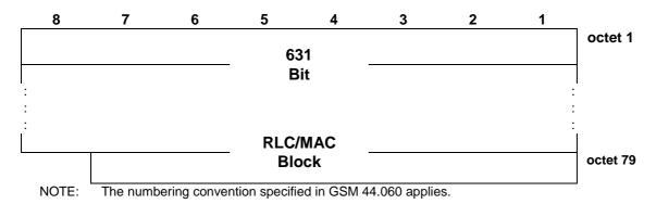
Figure 7.6.10.1: PDTCH block type 10 (MCS-6) uplink format
