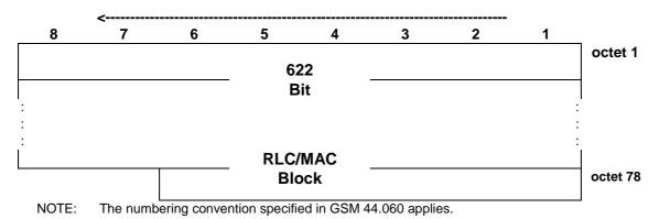
Figure 7.6.10.2: PDTCH block type 10 (MCS-6) downlink format
