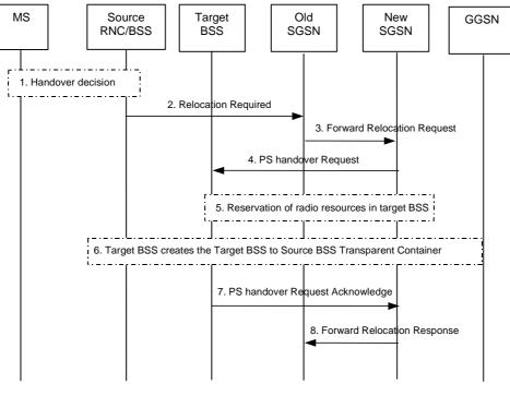
Figure 17: PS Handover Preparation Phase; Inter-RAT/mode, Inter-SGSN case (UTRAN/GERAN Iu mode  $\rightarrow$  GERAN A/Gb mode)
