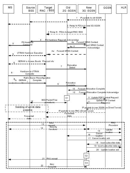
Figure 14: PS Handover Execution Phase; Inter-RAT/mode, Inter-SGSN case (GERAN A/Gb  $mode \rightarrow$  UTRAN/GERAN lu mode)
