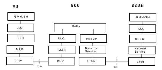
Figure 3: Control Plane Architecture in A/Gb mode
