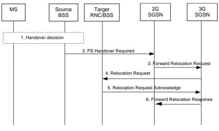
Figure 13: PS Handover Preparation Phase; Inter-RAT/mode, Inter-SGSN case (GERAN A/Gb mode  $\rightarrow$  UTRAN, GERAN lu mode)
