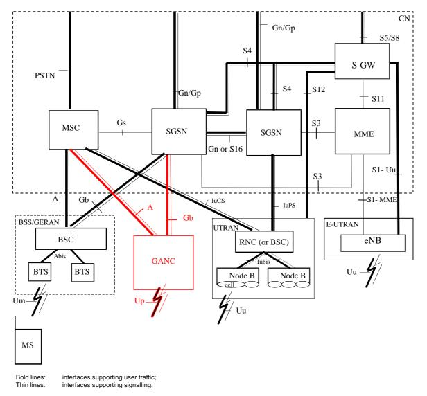
NOTE 1: The Iu interface is also supported by a GERAN BSS supporting Iu mode. NOTE 2: If both SGSNs support S4 interface then it is S16 otherwise Gn
