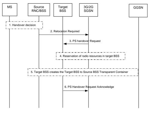
Figure 15: PS Handover Preparation Phase; Inter-RAT/mode, Intra-SGSN case (UTRAN/GERAN Iu mode  $\rightarrow$  GERAN A/Gb mode)
