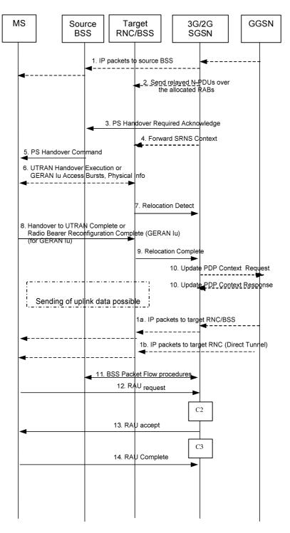
Figure 12: PS Handover Execution Phase; Inter-RAT/mode, Intra-SGSN case (GERAN A/Gb mode  $\rightarrow$  UTRAN, GERAN lu mode)
