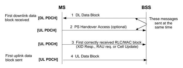
Figure 25: Option 2 - Blind Transmission in target cell, Synchronous Networks
