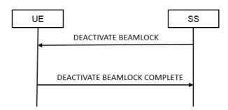
Figure 5.4.1-2: UE Beamlock test mode deactivation procedure
