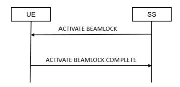
Figure 5.4.1-1: UE Beamlock test mode activation procedure
