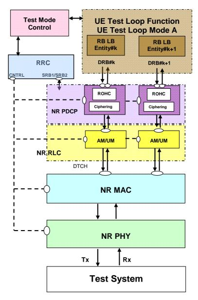
Figure 5.3.4.1-3: Model for Test Mode Control and UE Test Loop Mode A on UE side when standalone NR is configured
