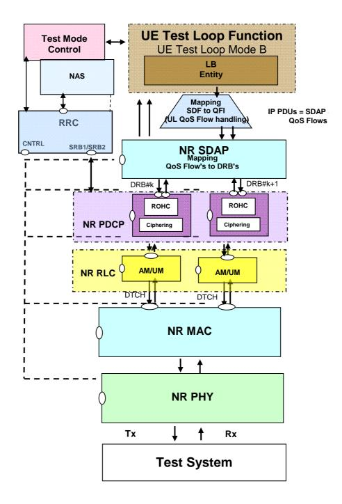
Figure 5.3.4.2.3-1: Model for Test Mode Control and UE Test Loop Mode B on UE side when standalone NR is configured
