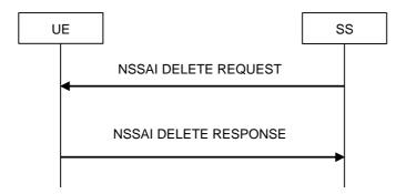
Figure 5.7.1-1: NSSAI delete test procedure
