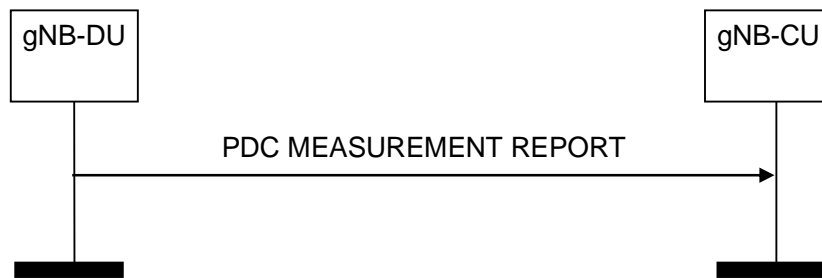
Figure 8.15.2.2-1: PDC Measurement Report procedure, successful operation
