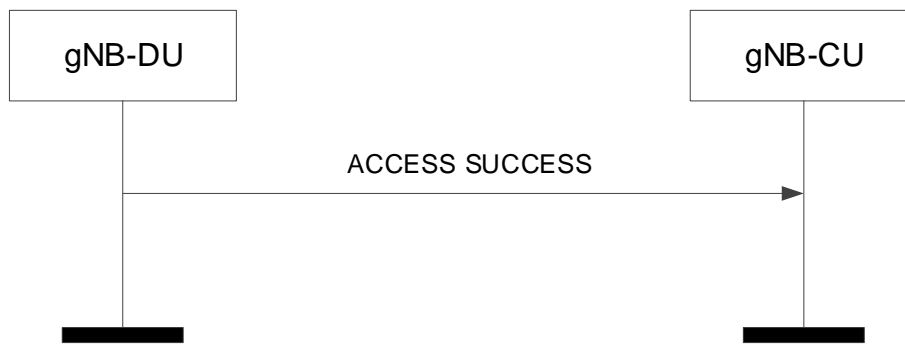
Figure 8.3.8.2-1: Access Success procedure. Successful operation.
