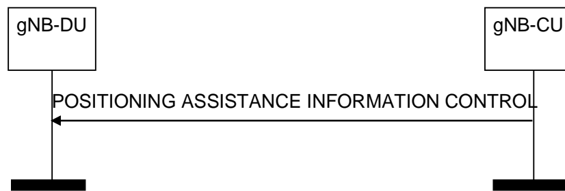
Figure 8.13.1.2-1: Positioning Assistance Information Control procedure
