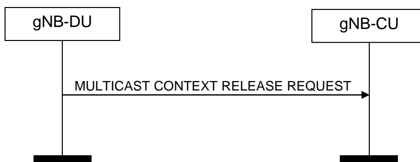
Figure 8.14.8.2-1: Multicast Context Release Request procedure. Successful operation
