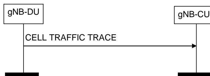
Figure 8.8.3.2-1: Cell Traffic Trace procedure. Successful operation.
