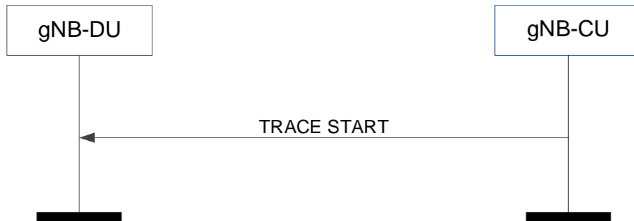
Figure 8.8.1.2-1: Trace start procedure: Successful Operation.
