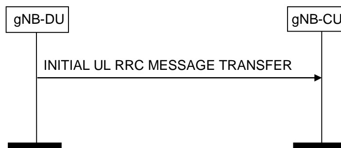
Figure 8.4.1.2-1: Initial UL RRC Message Transfer procedure.
