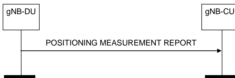
Figure 8.13.4.2-1: Positioning Measurement Report procedure: successful operation
