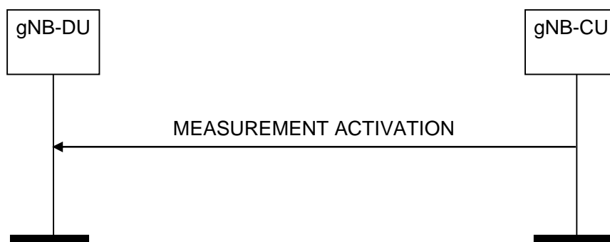
Figure 8.13.19.2-1: Measurement Activation procedure, successful operation
