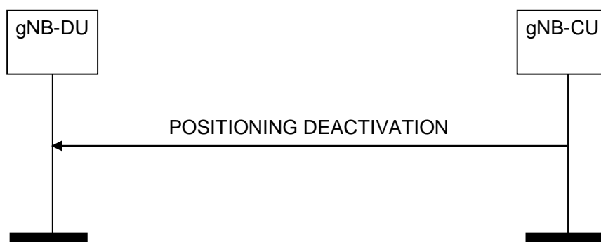
Figure 8.13.11.2-1: Positioning Deactivation procedure, successful operation
