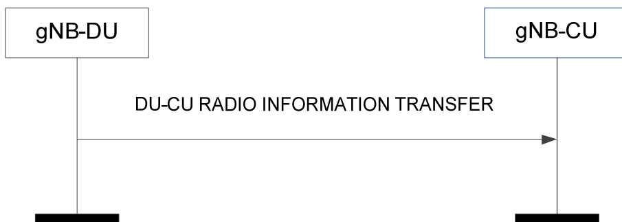
Figure 8.9.1.2-1: DU-CU Radio Information Transfer procedure.
