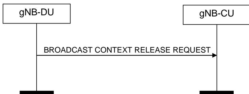
Figure 8.14.3.2-1: Broadcast Context Release Request procedure. Successful operation
