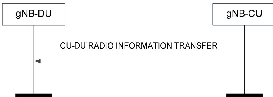
Figure 8.9.2.2-1: CU-DU Radio Information Transfer procedure.
