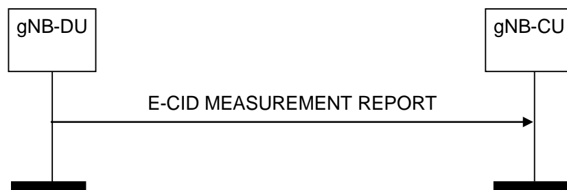
Figure 8.13.14.2-1: E-CID Measurement Report procedure, successful operation
