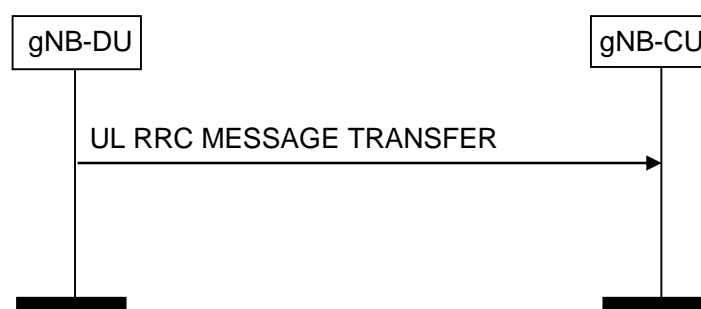
Figure 8.4.3.2-1: UL RRC Message Transfer procedure
