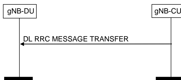
Figure 8.4.2.2-1: DL RRC Message Transfer procedure
