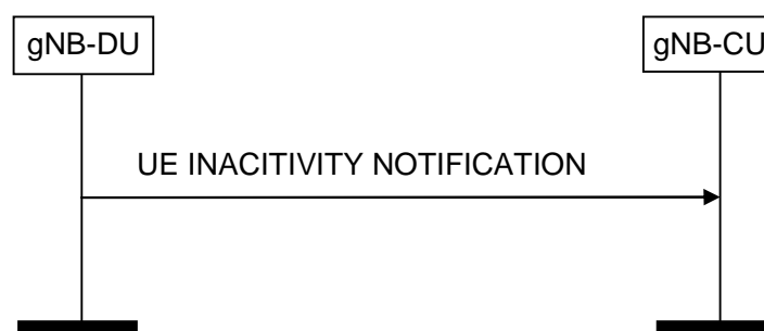
Figure 8.3.6.2-1: UE Inactivity Notification procedure.
