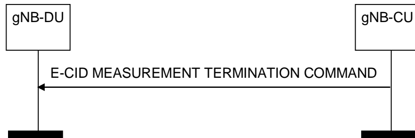
Figure 8.13.15.2-1: E-CID Measurement Termination procedure, successful operation
