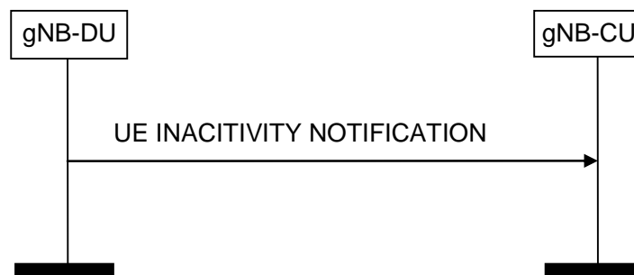
Figure 8.3.6.2-1: UE Inactivity Notification procedure.
