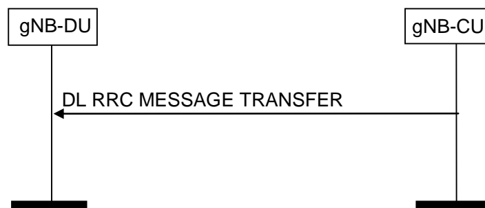
Figure 8.4.2.2-1: DL RRC Message Transfer procedure
