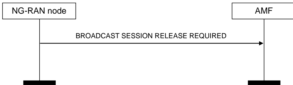
Figure 8.17.4.2-1: Broadcast Session Release Required, successful operation.
