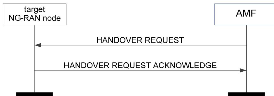
Figure 8.4.2.2-1: Handover resource allocation: successful operation
