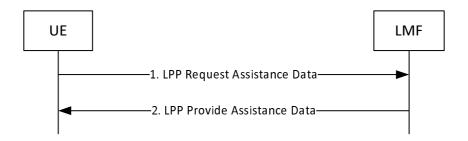
Figure 8.1.3.2.2-1: UE-initiated Assistance Data Transfer Procedure
