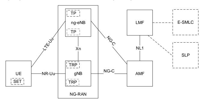
Figure 5.1-1: UE Positioning Overall Architecture applicable to NG-RAN
