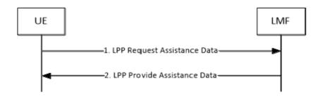
Figure 8.12.3.1.2.2-1: UE-initiated Assistance Data Transfer Procedure
