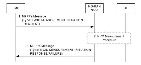
Figure 8.3.4.3.1-1: LMF-initiated Position Measurement Procedure
