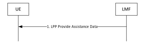
Figure 8.5.3.2.1: LMF-initiated Assistance Data Delivery Procedure
