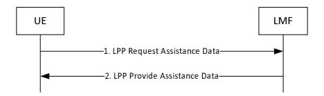
Figure 8.2.3.2.1.2-1: UE-initiated Assistance Data Transfer Procedure
