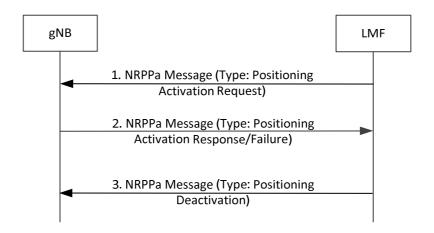
Figure 8.14.3.3a-1: Positioning Activation/Deactivation Procedure.
