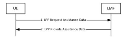
Figure 8.11.3.1.2.2-1: UE-initiated Assistance Data Transfer Procedure
