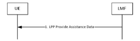
Figure 8.10.3.1.2.1.1-1: LMF-initiated Assistance Data Delivery Procedure
