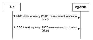
Figure 7.4.2.1-1: Inter-frequency RSTD measurement indication procedure
