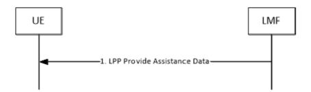
Figure 8.11.3.1.2.1-1: LMF-initiated Assistance Data Delivery Procedure
