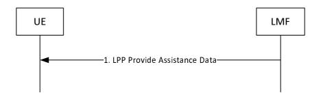
Figure 8.7.3.2.1-1: LMF-initiated Assistance Data Delivery Procedure
