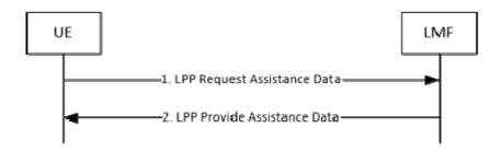
Figure 8.10.3.1.2.1.2-1: UE-initiated Assistance Data Transfer Procedure
