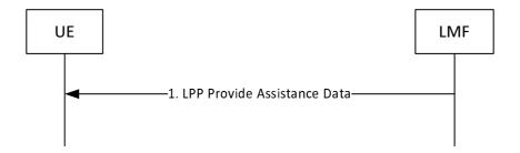
Figure 8.1.3.2.1-1: LMF-initiated Assistance Data Delivery Procedure
