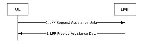
Figure 8.4.3.2.2-1: UE-initiated Assistance Data Transfer Procedure
