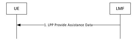
Figure 8.4.3.2.1-1: LMF-initiated Assistance Data Delivery Procedure
