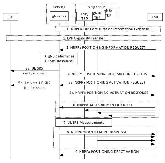
Figure 8.14.3.4-1: UL-AoA positioning procedure
