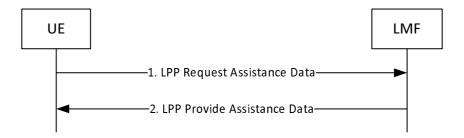
Figure 8.5.3.2.2-1: UE-initiated Assistance Data Transfer Procedure
