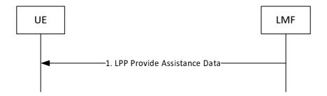
Figure 8.2.3.2.1.1-1: LMF-initiated Assistance Data Delivery Procedure
