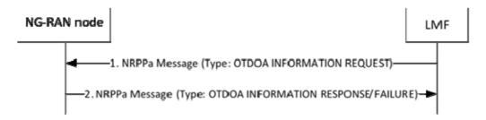
Figure 8.2.3.2.2.1-1: LMF-initiated Assistance Data Delivery Procedure
