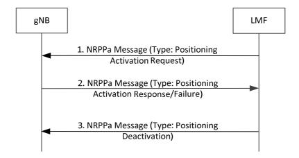
Figure 8.10.3.2.3-1: Positioning Activation/Deactivation Procedure.
