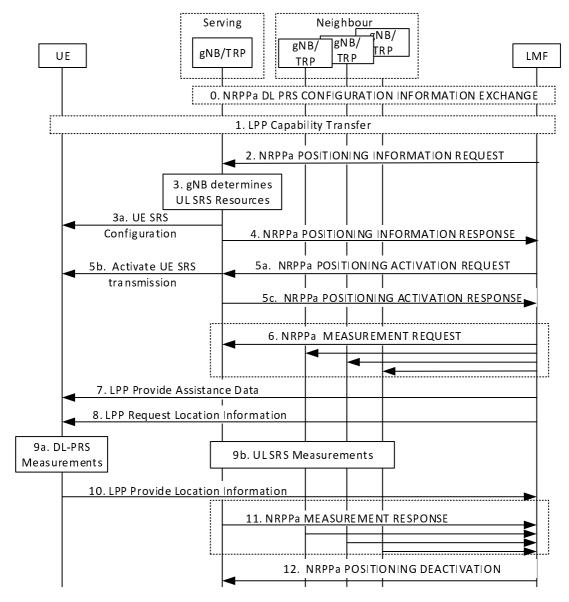
Figure 8.10.4-1: Multi-RTT positioning procedure
