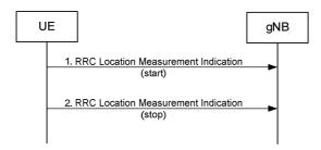
Figure 7.4.1.1-1: Location measurement indication procedure
