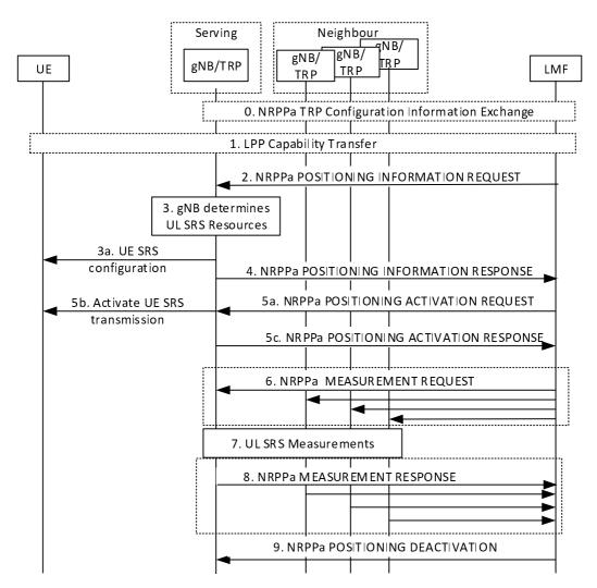
Figure 8.13.3.4-1: UL-TDOA positioning procedure
