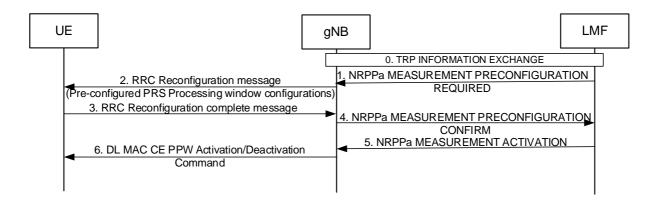
Figure 7.8.2-1: Pre-configured PRS processing window configuration procedure
