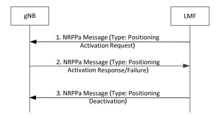
Figure 8.13.3.3a-1: Positioning Activation/Deactivation Procedure.
