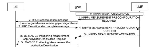
Figure 7.7.2-1: Pre-configured measurement gap configuration procedure
