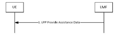
Figure 8.12.3.1.2.1-1: LMF-initiated Assistance Data Delivery Procedure
