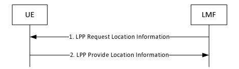
Figure 8.3.3.3-1: LMF-initiated Location Information Transfer Procedure.
