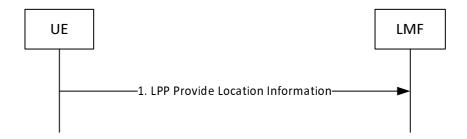
Figure 8.1.3.3.2-1: UE-initiated Location Information Delivery Procedure
