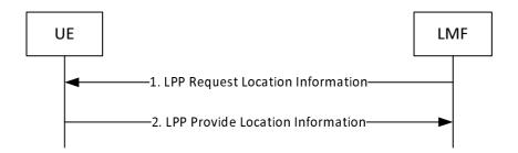
Figure 8.5.3.3.1-1: LMF-initiated Location Information Transfer Procedure
