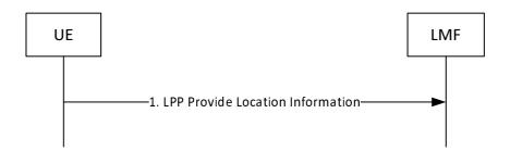
Figure 8.5.3.3.2-1: UE-initiated Location Information Delivery Procedure
