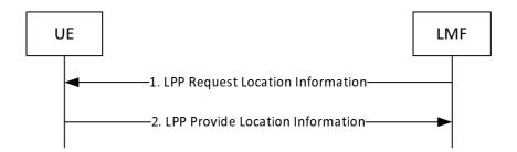
Figure 8.2.3.3.1-1: LMF-initiated Location Information Transfer Procedure
