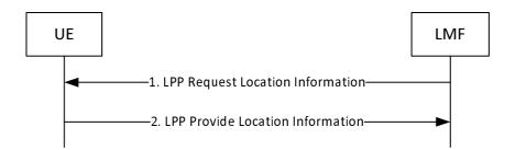
Figure 8.7.3.3.1-1: LMF-initiated Location Information Transfer Procedure
