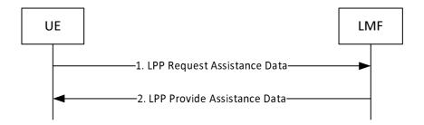
Figure 8.1.3.2.2-1: UE-initiated Assistance Data Transfer Procedure
