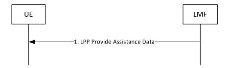
Figure 8.1.3.2.1-1: LMF-initiated Assistance Data Delivery Procedure
