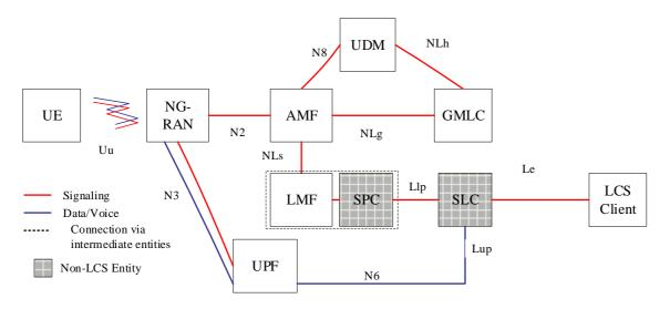
Figure A.2-1: System reference architecture reference for Location Services in reference point representation
