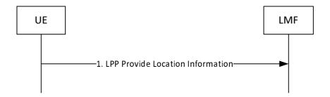
Figure 8.4.3.3.2-1: UE-initiated Location Information Delivery Procedure
