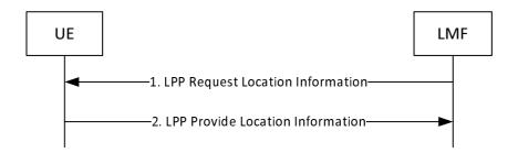
Figure 8.4.3.3.1-1: LMF-initiated Location Information Transfer Procedure
