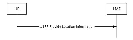
Figure 8.2.3.3.2-1: UE-initiated Location Information Delivery Procedure.
