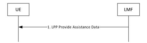
Figure 8.7.3.2.1-1: LMF-initiated Assistance Data Delivery Procedure
