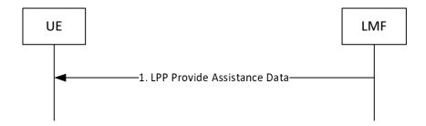
Figure 8.5.3.2.1: LMF-initiated Assistance Data Delivery Procedure
