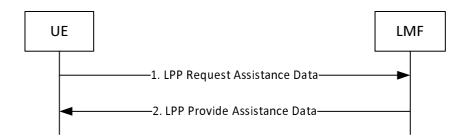
Figure 8.2.3.2.1.2-1: UE-initiated Assistance Data Transfer Procedure
