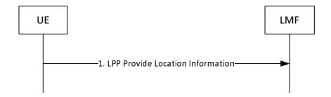
Figure 8.6.3.3.2-1: UE-initiated Location Information Delivery Procedure
