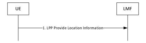
Figure 8.7.3.3.2-1: UE-initiated Location Information Delivery Procedure
