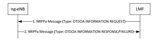
Figure 8.2.3.2.2.1-1: LMF-initiated Assistance Data Delivery Procedure
