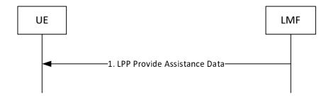
Figure 8.2.3.2.1.1-1: LMF-initiated Assistance Data Delivery Procedure
