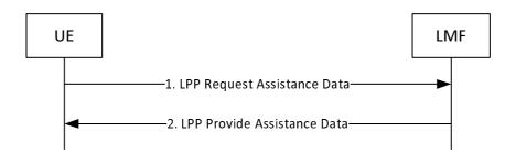
Figure 8.4.3.2.2-1: UE-initiated Assistance Data Transfer Procedure
