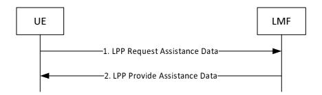
Figure 8.5.3.2.2-1: UE-initiated Assistance Data Transfer Procedure
