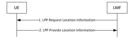
Figure 8.1.3.3.1-1: LMF-initiated Location Information Transfer Procedure
