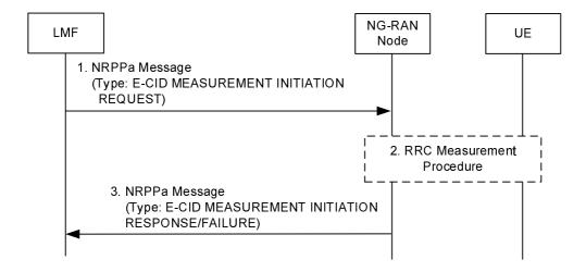
Figure 8.3.4.3.1-1: LMF-initiated Position Measurement Procedure
