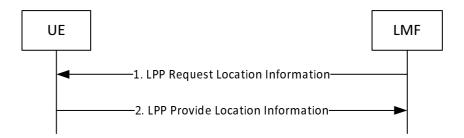
Figure 8.6.3.3.1-1: LMF-initiated Location Information Transfer Procedure
