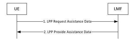
Figure 8.7.3.2.2-1: UE-initiated Assistance Data Transfer Procedure
