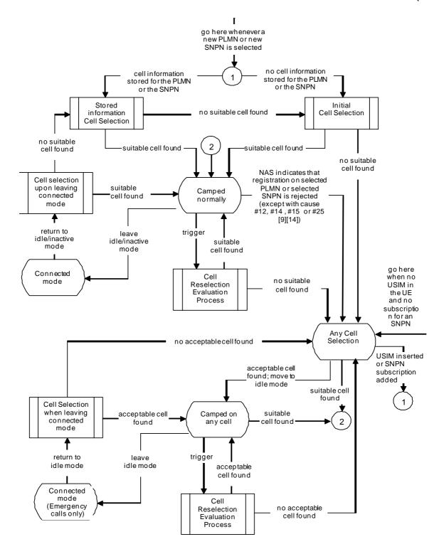
Figure 5.2.2-1: RRC\_IDLE and RRC\_INACTIVE Cell Selection and Reselection
