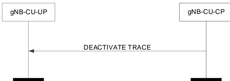
Figure 8.4.2.2-1: Deactivate trace procedure: Successful Operation.
