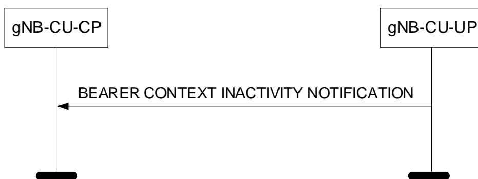
Figure 8.3.6.2-1: Bearer Context Inactivity Notification procedure: Successful Operation.
