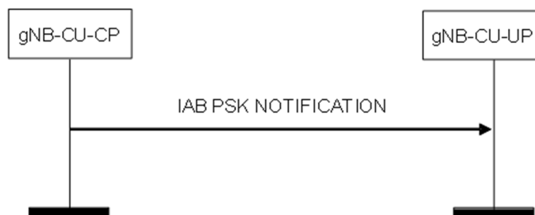
Figure 8.5.2.2-1: IAB PSK Notification procedure: Successful Operation.
