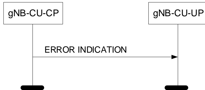
Figure 8.2.2.2-1: Error Indication procedure, gNB-CU-CP originated. Successful operation.
