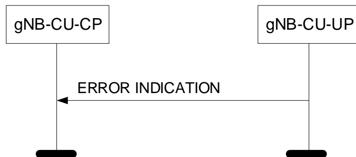
Figure 8.2.2.2-2: Error Indication procedure, gNB-CU-UP originated. Successful operation.
