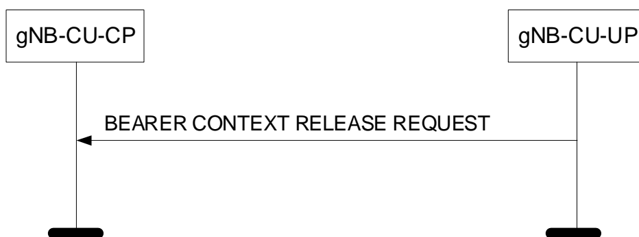
Figure 8.3.5.2-1: Bearer Context Release Request procedure: Successful Operation.
