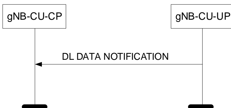
Figure 8.3.7.2-1: DL Data Notification procedure: Successful Operation.
