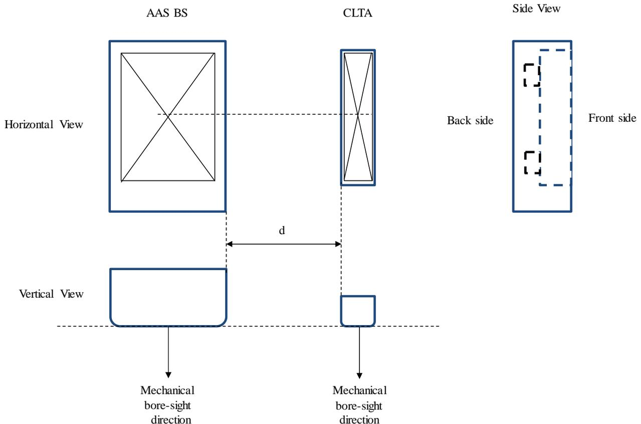
Figure 4.15.2.3-1 Alignment of AAS BS and CLTA
