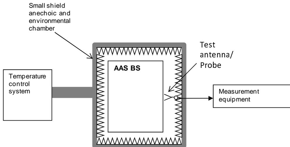
**Figure F.7.2-1: Measurement set up for Extreme conditions for EIRP accuracy using difference method**
