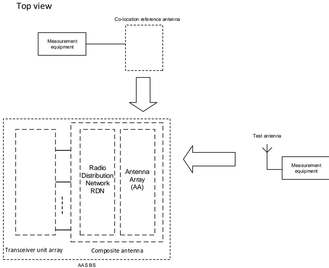
Figure 4.8.2-2: Receiver test interfaces for co-location concept
