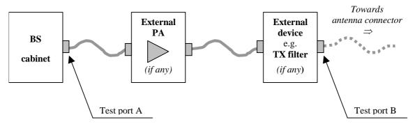
Figure 4.10.1-1: Transmitter test ports
