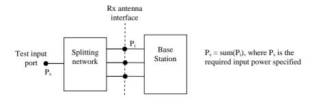
Figure 4.10.7.1-1: Receiver test set-up
