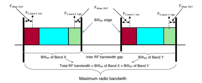
Figure 3.2-3: Illustration of Maximum Radio Bandwidth and Total RF Bandwidth for Multi-band Multistandard Radio
