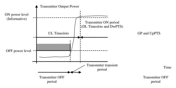
Figure 6.4.1-1: Illustration of the relations of transmitter ON period, transmitter OFF period and transmitter transient period (for E-UTRA/UTRA)
