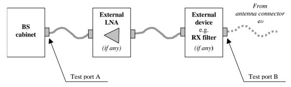
Figure 4.10.2-1: Receiver test ports
