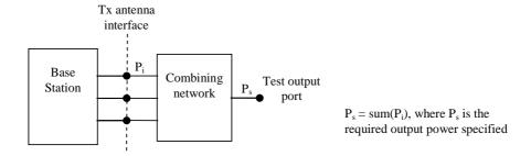
Figure 4.10.7.2-1: Transmitter test set-up
