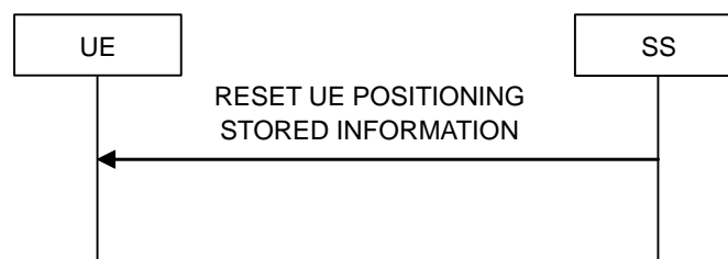
Figure 5.5.1-1: Reset UE Positioning Stored Information procedure
