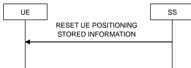
Figure 5.5.1-1: Reset UE Positioning Stored Information procedure
