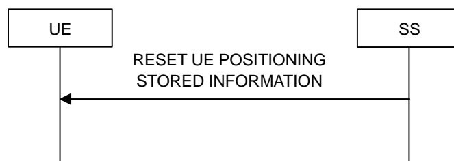
Figure 5.5.1-1: Reset UE Positioning Stored Information procedure
