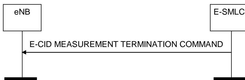
Figure 8.2.4.2-1: E-CID Measurement Termination procedure, successful operation
