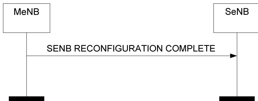
**Figure 8.6.2.2-1: SeNB Reconfiguration Complete procedure, successful operation.**
