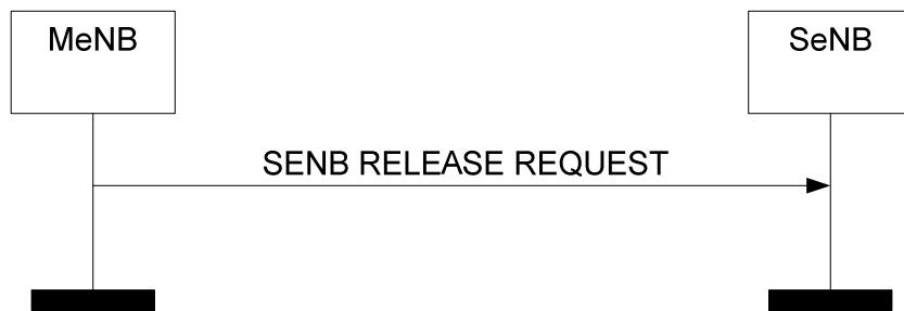
**Figure 8.6.5.2-1: MeNB initiated SeNB Release, successful operation**
