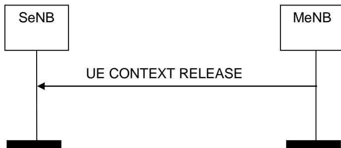
**Figure 8.2.3.2-2: UE Context Release, successful operation for dual connectivity**
