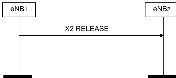
**Figure 8.4.2-1: X2AP Release, successful operation**
