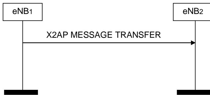
**Figure 8.5.2-1: X2AP Message Transfer, successful operation**
