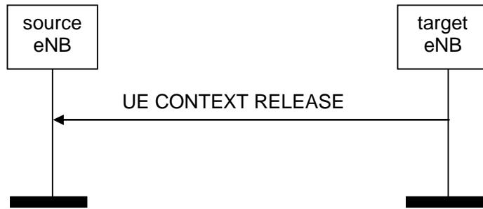
**Figure 8.2.3.2-1: UE Context Release, successful operation for handover**
