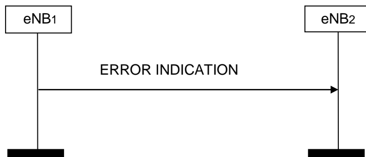
Figure 8.3.2.2-1: Error Indication, successful operation.
