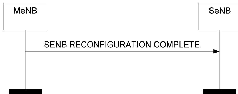
Figure 8.6.2.2-1: SeNB Reconfiguration Complete procedure, successful operation.
