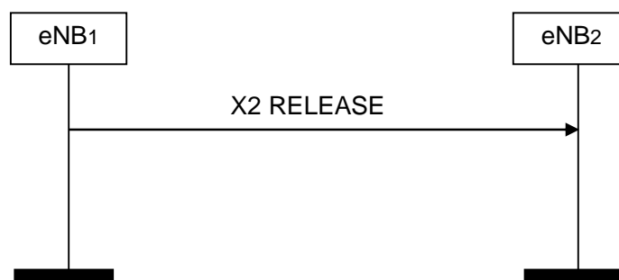
Figure 8.4.2-1: X2AP Release, successful operation
