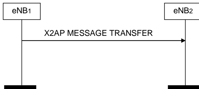
Figure 8.5.2-1: X2AP Message Transfer, successful operation
