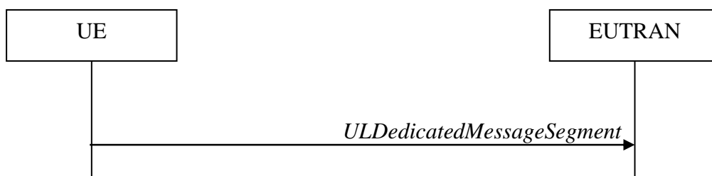
Figure 5.6.22.1-1: UL message segment transfer
