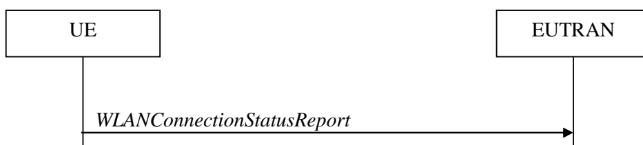
Figure 5.6.15.2.1-1: WLAN connection status reporting
