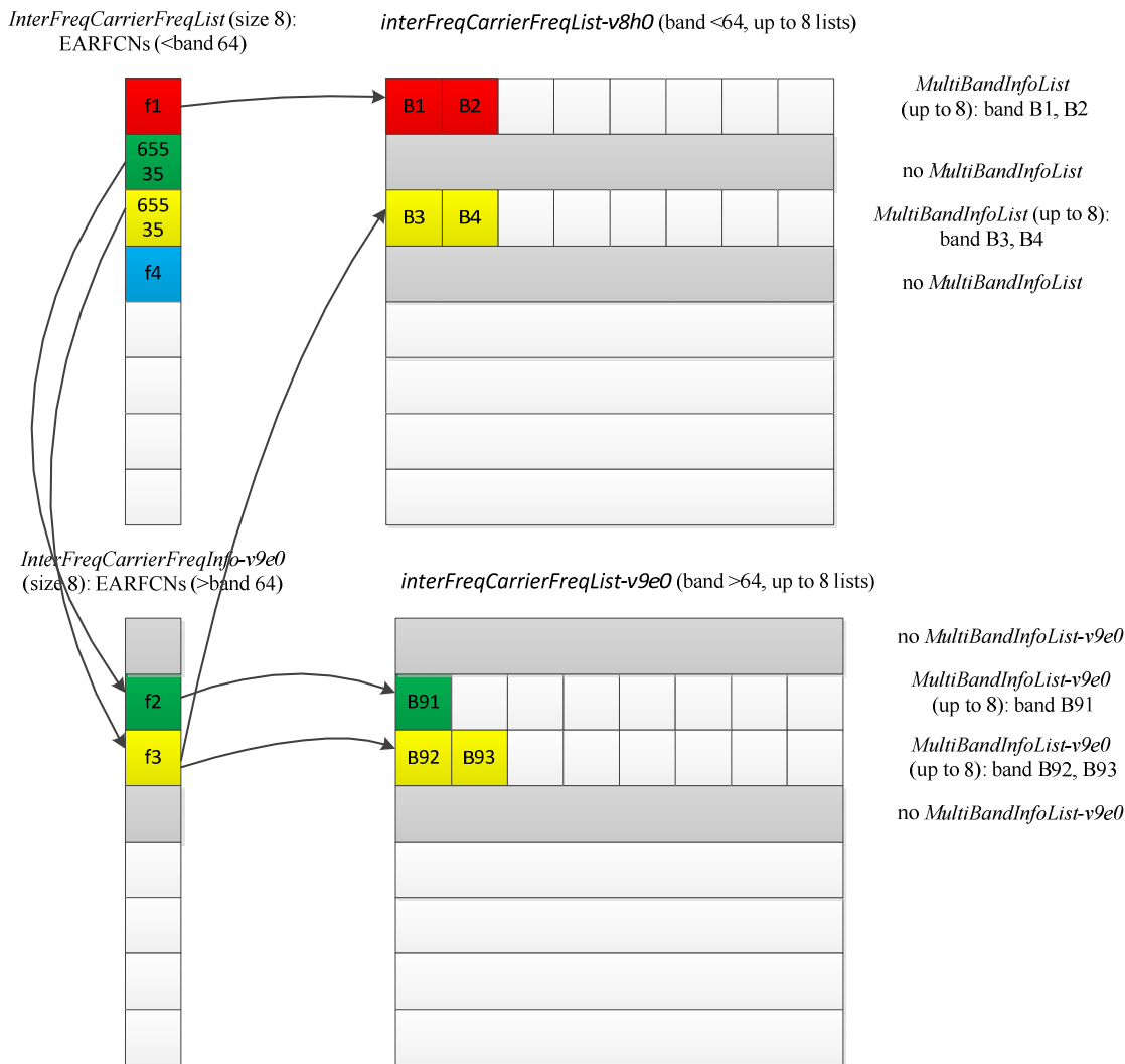
Figure D.1.2-1: Mapping of EARFCNs to MultiBandInfoList/MultiBandInfoList-v9e0
