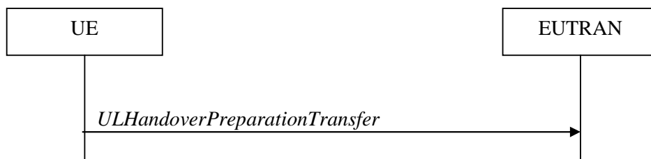
Figure 5.4.5.1-1: UL handover preparation transfer
