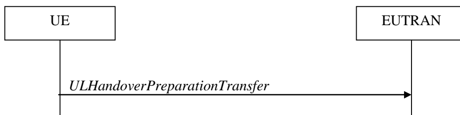
Figure 5.4.5.1-1: UL handover preparation transfer
