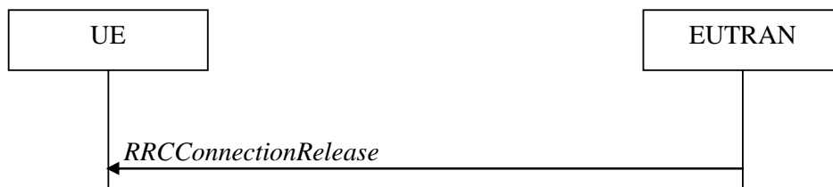
Figure 5.3.8.1-1: RRC connection release, successful
