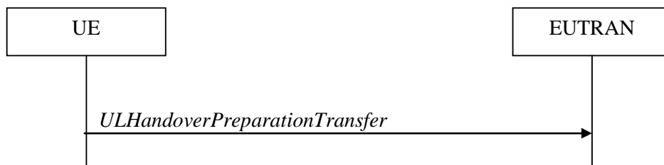
Figure 5.4.5.1-1: UL handover preparation transfer
