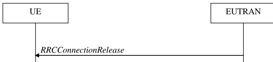
Figure 5.3.8.1-1: RRC connection release, successful
