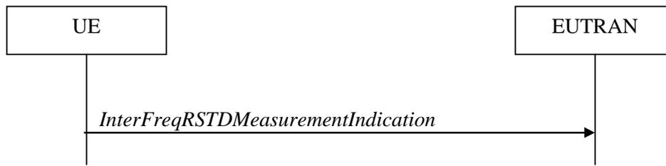
**Figure 5.5.7.1-1: Inter-frequency RSTD measurement indication**
