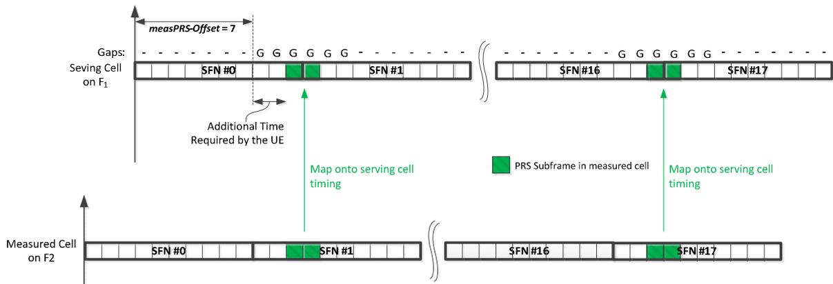
Figure 6.2.2-1 (informative): Exemplary calculation of *measPRS-Offset* field.
