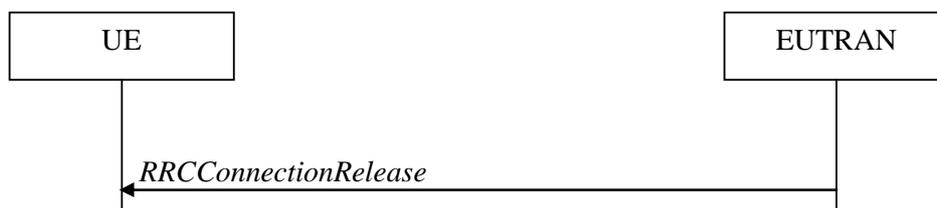
**Figure 5.3.8.1-1: RRC connection release, successful**
