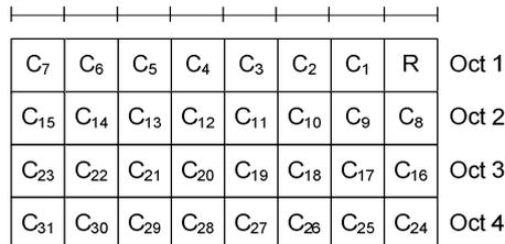
**Figure 6.1.3.8-2: Activation/Deactivation MAC control element of four octets**
