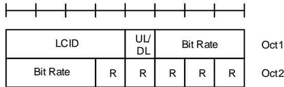
Figure 6.1.3.13-1: Recommended bit rate MAC control element
