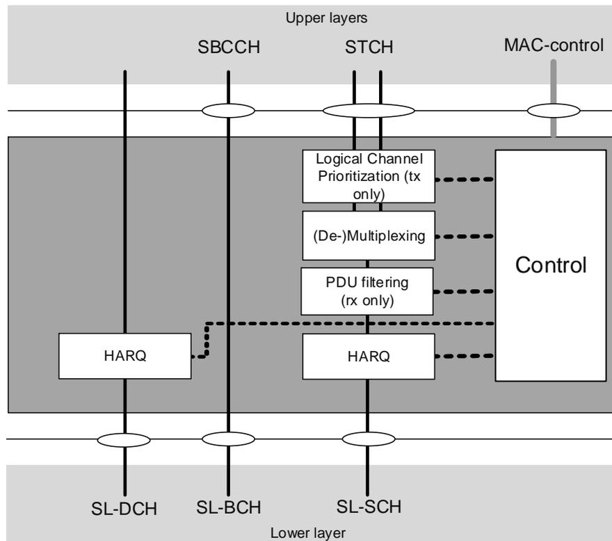
Figure 4.2.1-3: MAC structure overview for sidelink, UE side
