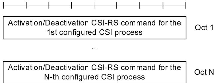
**Figure 6.1.3.14-1: Activation/Deactivation of CSI-RS resources MAC Control Element**
