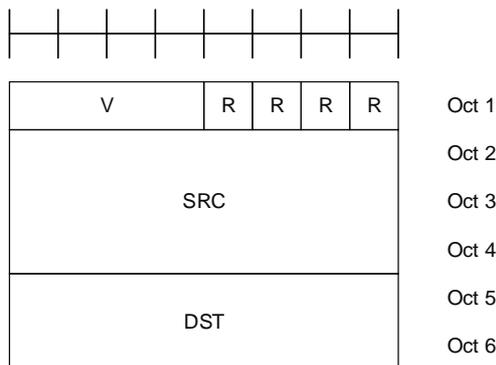
Figure 6.1.6-3: SL-SCH MAC subheader for V = "0001" and "0010"
