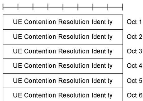
**Figure 6.1.3.4-1: UE Contention Resolution Identity MAC control element**
