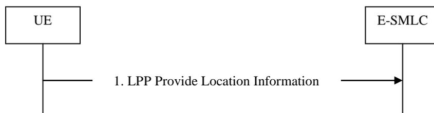
**Figure 8.6.3.2-1: UE-initiated Location Information Delivery Procedure**
