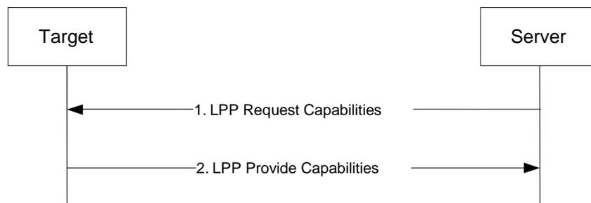
**Figure 7.1.2.1-1: LPP Capability Transfer procedure**
