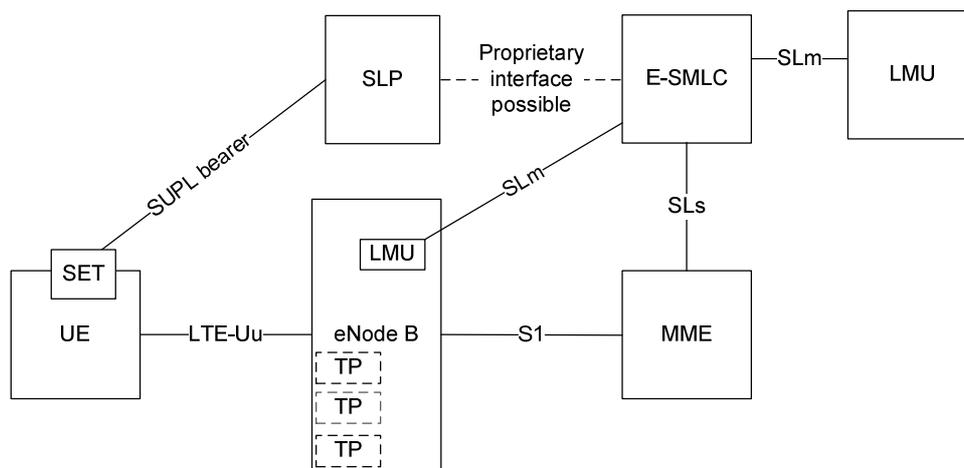
**Figure 5-1: UE Positioning Architecture applicable to E-UTRAN**
