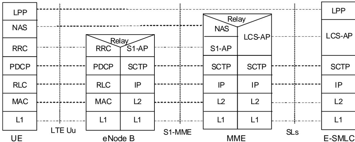
Figure 6.4.1-1: Protocol Layering for E-SMLC to UE Signalling
