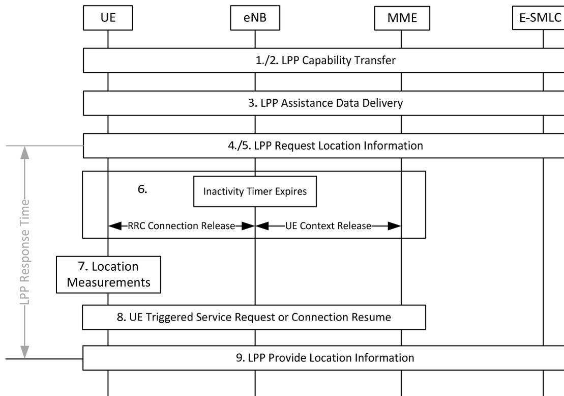
**Figure 7.1.3-1: UE positioning measurements in idle state.**
