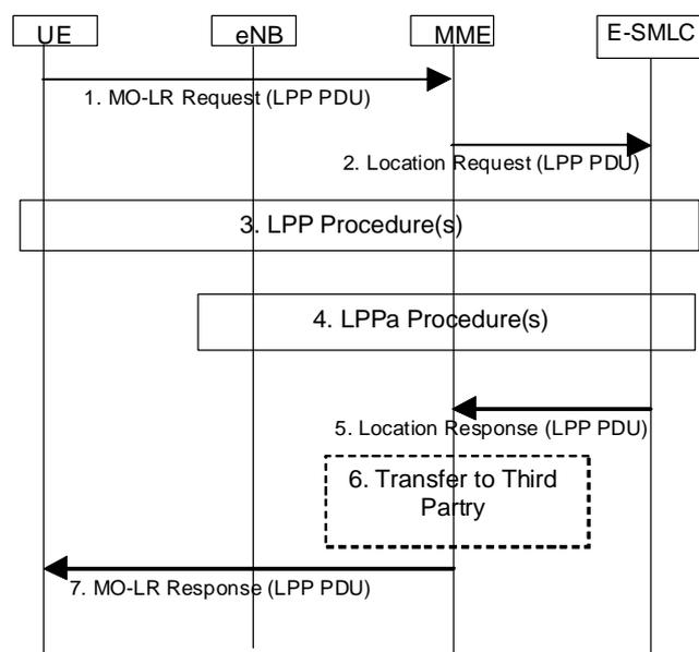
**Figure 7.3.2-1: UE Positioning Operations to support an MO-LR**
