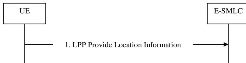
**Figure 8.8.3.1.2-1: UE-initiated Location Information Delivery Procedure**
