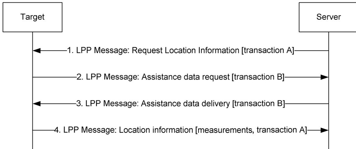
**Figure 7.1.2.4-1: Example of multiple LPP procedures**
