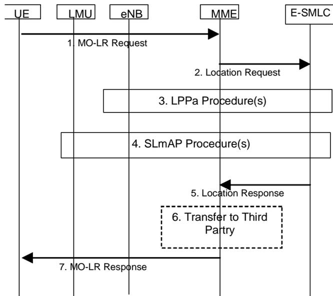
**Figure 7.5.2-1: UE Positioning Operations to support an MO-LR**
