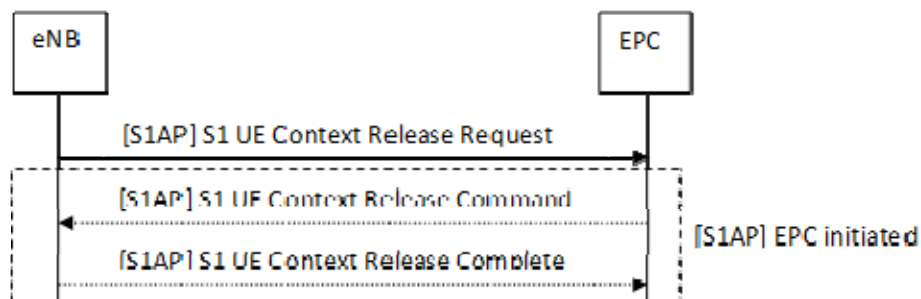
Figure 19.2.2.2.2-1: S1 UE Context Release Request procedure (eNB triggered) and subsequent S1 UE Context Release procedure (EPC triggered)
