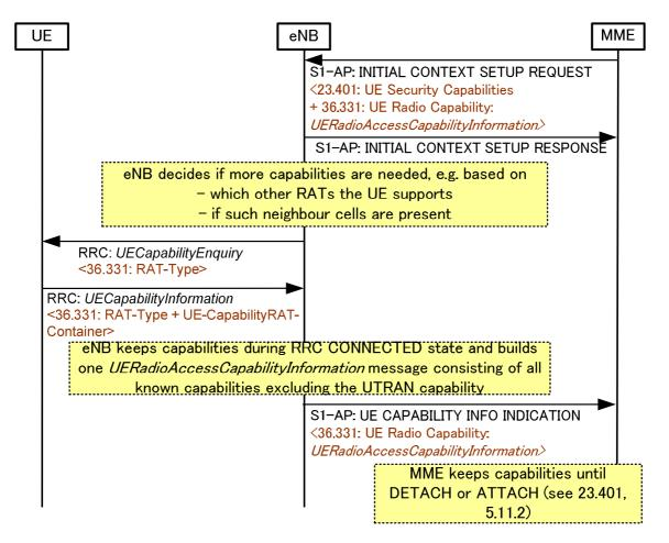
Figure 18-1: Initial UE Capability Handling
