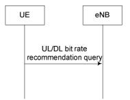
Figure 23.15.1-2: UL or DL bit rate recommendation query
