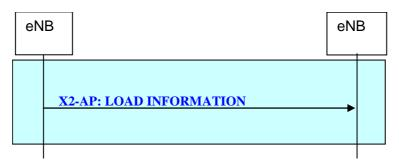
Figure 20.2.2.6-1: Load Indication procedure
