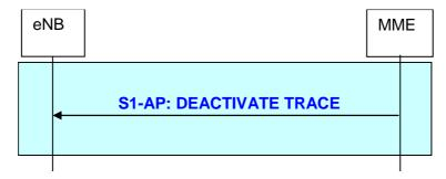
Figure 19.2.2.19.3-1: Deactivate Trace procedure
