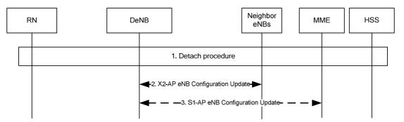
Figure 4.7.6.4-1: RN detach procedure
