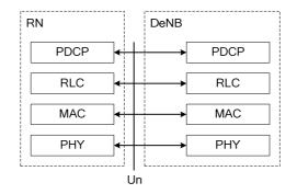
Figure 4.7.5-2: Radio user plane protocol stack for supporting RNs
