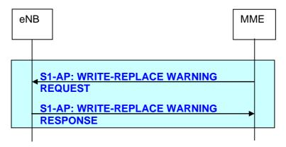
Figure 19.2.2.13.1-1: Write-Replace Warning procedure
