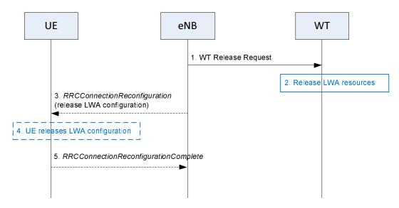
Figure 22A.1.7.3-1: WT Release procedure -eNB initiated
