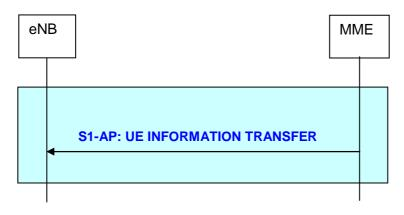
Figure 19.2.2.29: UE Information Transfer procedure
