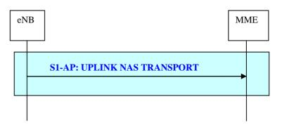
Figure 19.2.2.6-2: Uplink NAS Transport procedure
