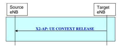
Figure 20.2.2.3-1: UE Context Release procedure for handover and DC.
