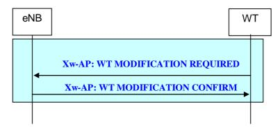
Figure 22B.2.2.4-1: WT initiated WT Modification procedure
