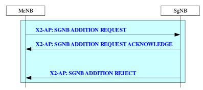
Figure 20.2.2.20-1: SgNB Addition Preparation procedure
