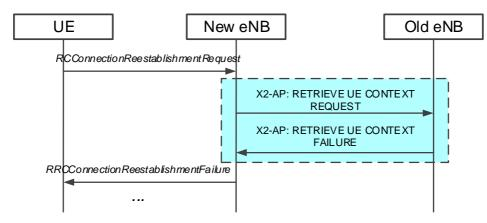
Figure 20.2.2.19-3: Retrieve UE Context procedure (highlighted in blue) for cases of UE reestablishment. Unsuccessful case
