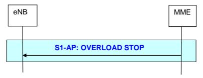
Figure 19.2.2.12.2-1: Overload Stop procedure
