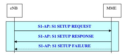
Figure 19.2.2.8-1: S1 Setup procedure
