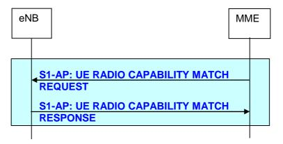
Figure 19.2.2.21-1: UE Radio Capability Match procedure
