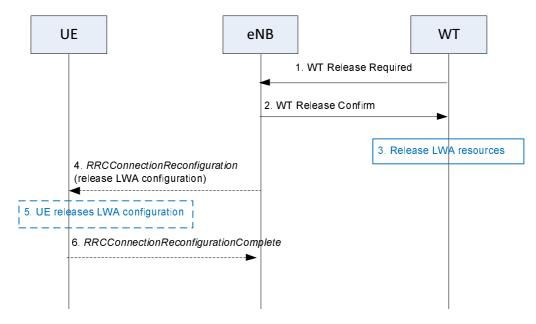
Figure 22A.1.7.3-2: WT Release procedure –WT initiated
