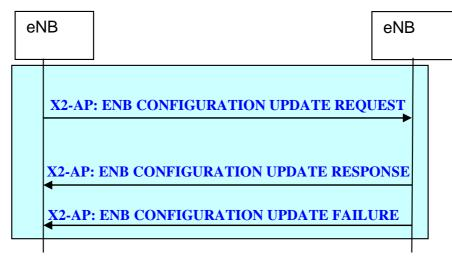
Figure 20.2.2.8-1: eNB Configuration Update procedure
