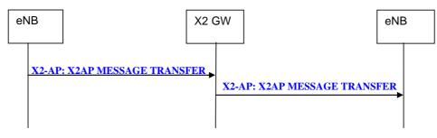
Figure 20.2.2.17-1: X2AP Message Transfer procedure
