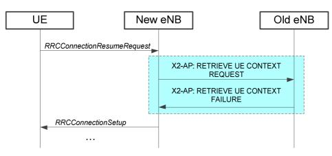
Figure 20.2.2.19-2: Retrieve UE Context procedure (highlighted in blue) for cases of UE context resumption. Unsuccessful case
