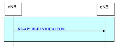
Figure 20.2.2.12-1: Radio Link Failure Indication procedure
