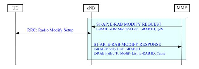
Figure 19.2.2.4.2-1: E-RAB Modification procedure
