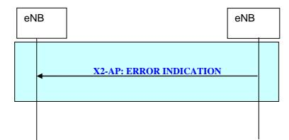
Figure 20.2.2.5-1: Error Indication procedure between eNB and eNB
