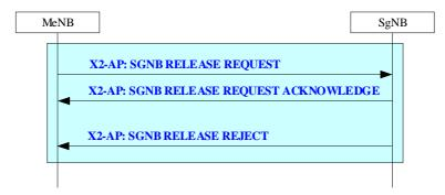
Figure 20.2.2.24-1: MeNB initiated SgNB Release procedure
