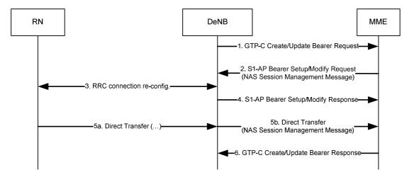
Figure 4.7.6.2-1: DeNB-initiated bearer activation/modification procedure
