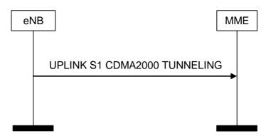
Figure 19.2.2.16.2-1: Uplink S1 CDMA2000 Tunnelling procedure
