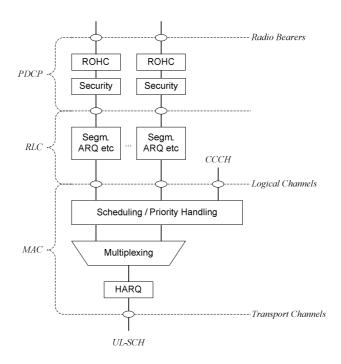
Figure 6-2: Layer 2 Structure for UL
