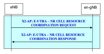
Figure 20.2.2.31-1: E-UTRA - NR Cell Resource Coordination procedure triggered by the eNB.
