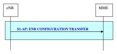
Figure 19.2.2.9a-1: eNB Configuration Transfer procedure
