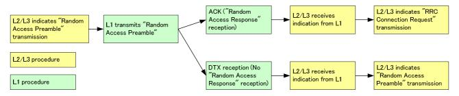
Figure 10.1.5.3-1: Interaction model between L1 and L2/3 for Random Access Procedure
