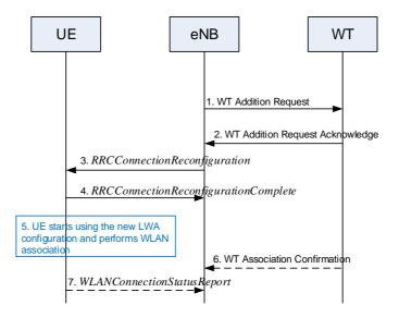
Figure 22A.1.7.1-1: WT Addition procedure
