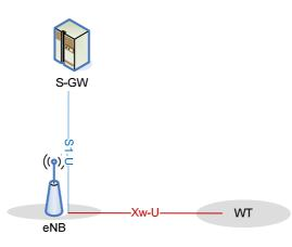
Figure 22A.1.3.2-1: U-Plane connectivity of eNB and WT for LWA
