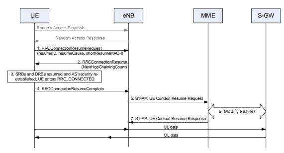
Figure 7.3a.3-2: RRC Connection Resume procedure
