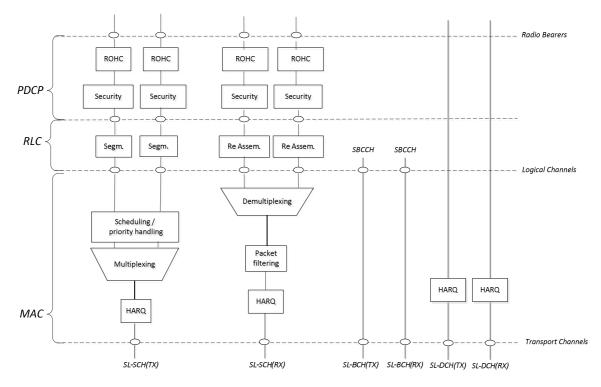
Figure 6-3: Layer 2 Structure for Sidelink
