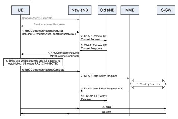
Figure 7.3a.3-3: RRC Connection Resume procedure in different eNB
