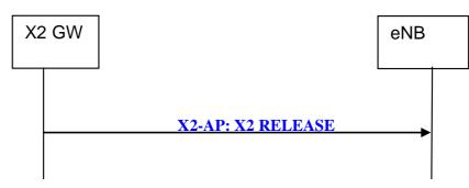
Figure 20.2.2.16-1: X2 Release procedure
