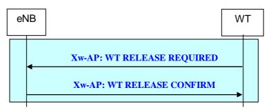
Figure 22B.2.2.6-1: WT initiated WT Release procedure
