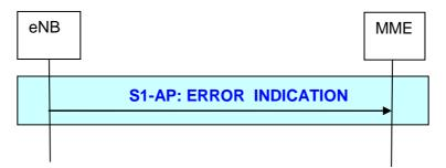
Figure 19.2.2.7.2a-1: eNB initiated Error Indication procedure
