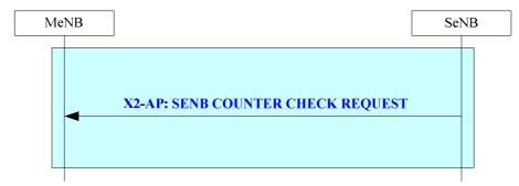
Figure 20.2.2.2g-1: SeNB Counter Check procedure
