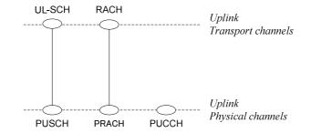
Figure 5.3.1-2: Mapping between uplink transport channels and uplink physical channels
