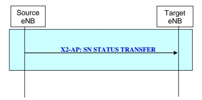
Figure 20.2.2.4-1: SN Status Transfer procedure for handover.
