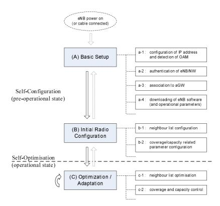
Figure 22.1-1: Ramifications of Self-Configuration /Self-Optimization functionality
