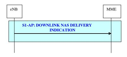
Figure 19.2.2.6-5: Downlink NAS Delivery Indication procedure
