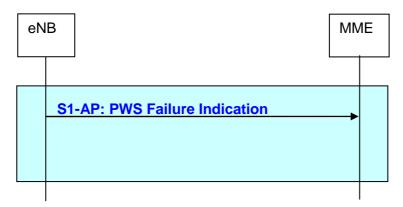
Figure 19.2.2.23-1: PWS Failure Indication procedure
