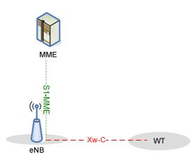
Figure 22A.1.3.3-1: C-Plane connectivity of eNB and WT for LWA
