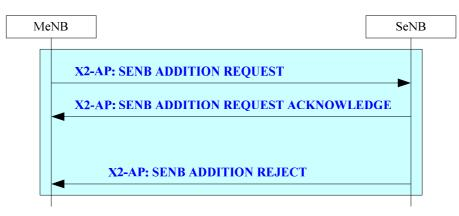
Figure 20.2.2.2a-1: SeNB Addition Preparation procedure
