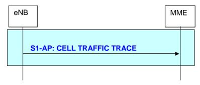
Figure 19.2.2.19.4-1: Cell Traffic Trace procedure
