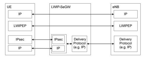
Figure 22A.3-3: Bearer over LWIP Tunnel - Protocol Stack
