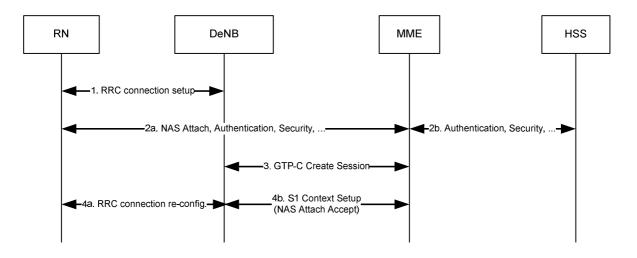
Figure 4.7.6.1-1: RN attach procedure
