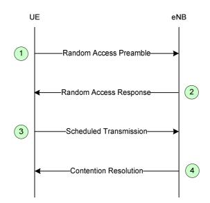
Figure 10.1.5.1-1: Contention based Random Access Procedure
