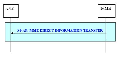
Figure 19.2.2.15-1: MME Direct Information Transfer procedure
