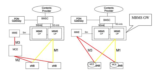
Figure 15.1.1-2: eMBMS Architecture deployment alternatives
