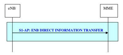
Figure 19.2.2.14-1: eNB Direct Information Transfer procedure
