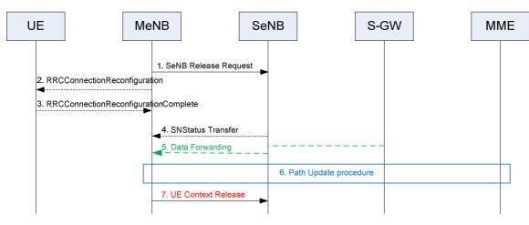
Figure 10.1.2.8.3-1: SeNB Release procedure – MeNB initiated
