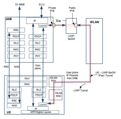
Figure 22A.3-2: LWIP Protocol Architecture
