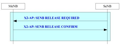
Figure 20.2.2.2f-1: SeNB initiated SeNB Release procedure
