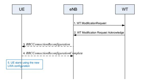
Figure 22A.1.7.2-1: WT Modification procedure – eNB initiated
