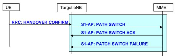
Figure 19.2.2.5.5-1: Path Switch procedure
