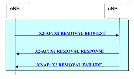
Figure 20.2.2.18-1: X2 Removal procedure
