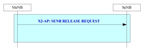
Figure 20.2.2.2e-1: MeNB initiated SeNB Release procedure
