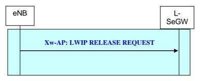
Figure 22B.2.2.15-1: eNB initiated LWIP-SeGW Release procedure
