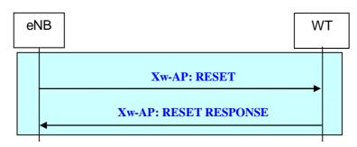
Figure 22B.2.2.12.2-1: Reset procedure initiated by eNB
