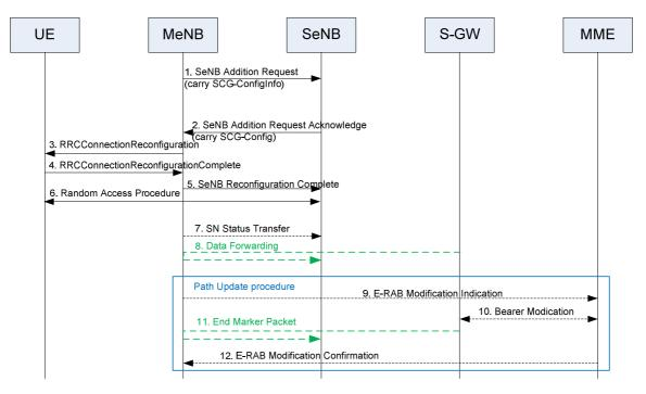
Figure 10.1.2.8.1-1: SeNB Addition procedure
