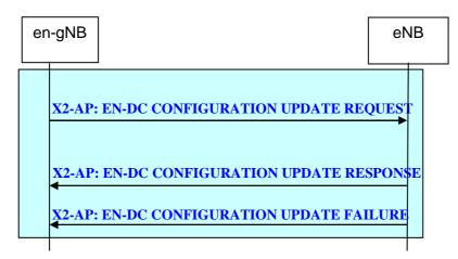
Figure 20.2.2.29-2: EN-DC Configuration Update procedure triggered by the en-gNB.
