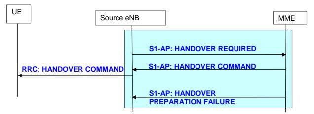
Figure 19.2.2.5.1-1: Handover preparation procedure
