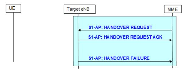
Figure 19.2.2.5.2-1: Handover resource allocation procedure
