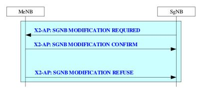
Figure 20.2.2.23-1: SgNB initiated SgNB Modification procedure
