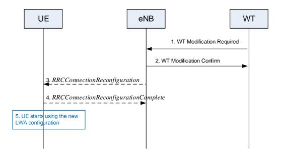
Figure 22A.1.7.2-2: WT Modification procedure – WT initiated
