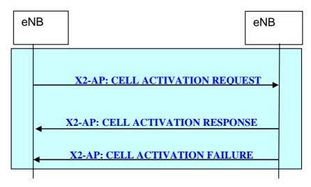
Figure 20.2.2.15-1: Cell Activation procedure
