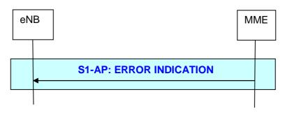
Figure 19.2.2.7.2b-1: MME initiated Error Indication procedure
