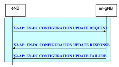
Figure 20.2.2.29-1: EN-DC Configuration Update procedure triggered by the eNB.
