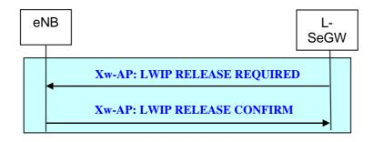
Figure 22B.2.2.16-1: LWIP-SeGW initiated LWIP-SeGW Release procedure
