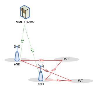
Figure 22A.1.1-1: Non-collocated LWA Overall Architecture
