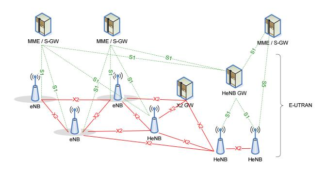
The overall E-UTRAN architecture with deployed HeNB GW and X2 GW is shown below.
