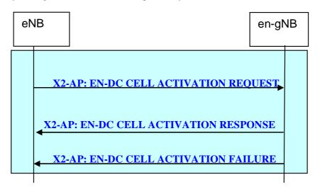
Figure 20.2.2.30-1: EN-DC Cell Activation procedure
