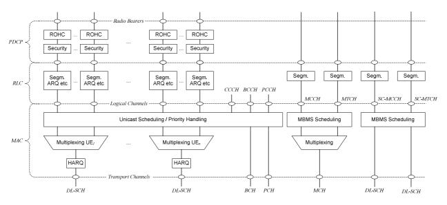
Figure 6-1: Layer 2 Structure for DL
