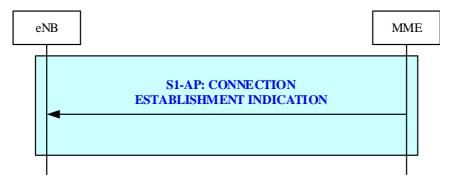
Figure 19.2.2.25-1: Connection Establishment Indication procedure
