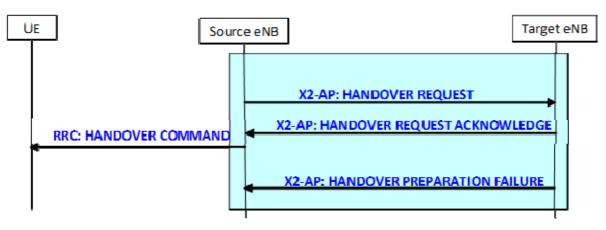
Figure 20.2.2.1-1: Handover Preparation procedure
