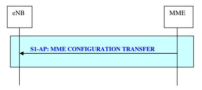
Figure 19.2.2.10a-1: MME Configuration Transfer procedure
