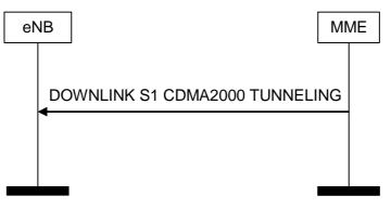
Figure 19.2.2.16.1-1: Downlink S1 CDMA2000 Tunnelling procedure
