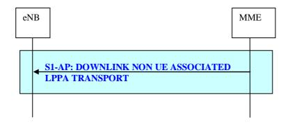
Figure 19.2.2.18.3-1: Downlink Non UE Associated LPPa Transport procedure
