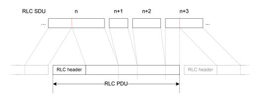
Figure 6.2.2-1: RLC PDU Structure
