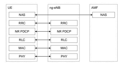
Figure 24.2.2-1: Control Plane Protocol Stack
