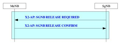
Figure 20.2.2.25-1: SgNB initiated SgNB Release procedure
