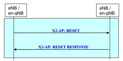
Figure 20.2.2.9-1: Reset procedure between eNBs
