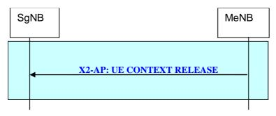
Figure 20.2.2.3-2: UE Context Release procedure for EN-DC.
