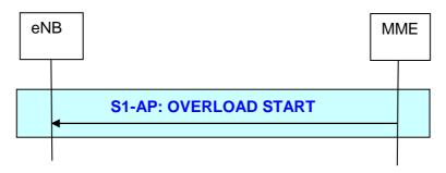
Figure 19.2.2.12.1-1 Overload Start procedure
