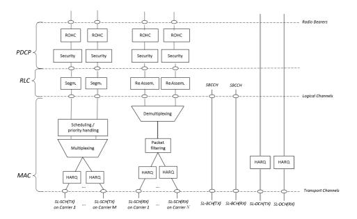
Figure 6.4-3: Layer 2 Structure for Sidelink with CA configured
