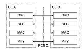
Figure 23.10.2.2-1: Control-Plane protocol stack for SBCCH
