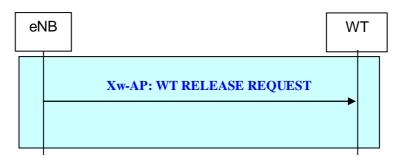
Figure 22B.2.2.5-1: eNB initiated WT Release procedure
