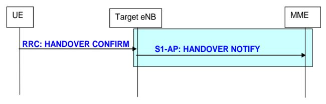
Figure 19.2.2.5.3-1: Handover completion procedure
