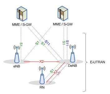
Figure 4.7.2-1: Overall E-UTRAN Architecture supporting RNs
