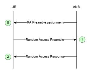
Figure 10.1.5.2-1: Non-contention based Random Access Procedure
