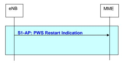
Figure 19.2.2.22-1: PWS Restart Indication procedure
