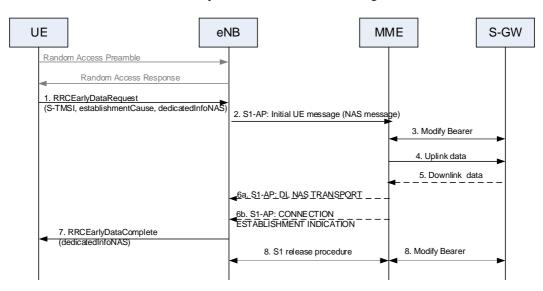
Figure 7.3b-1: EDT for Control Plane CIoT EPS Optimizations
