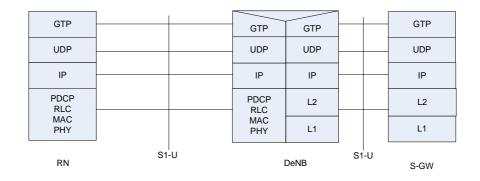
Figure 4.7.3-1: S1 user plane protocol stack for supporting RNs
