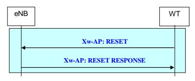
Figure 22B.2.2.12.1-1: Reset procedure initiated by WT
