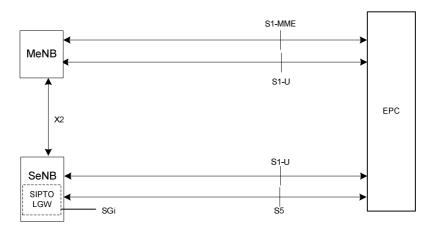
Figure 4.9.3.4-2: SIPTO@LN with co-located L-GW in SeNB
