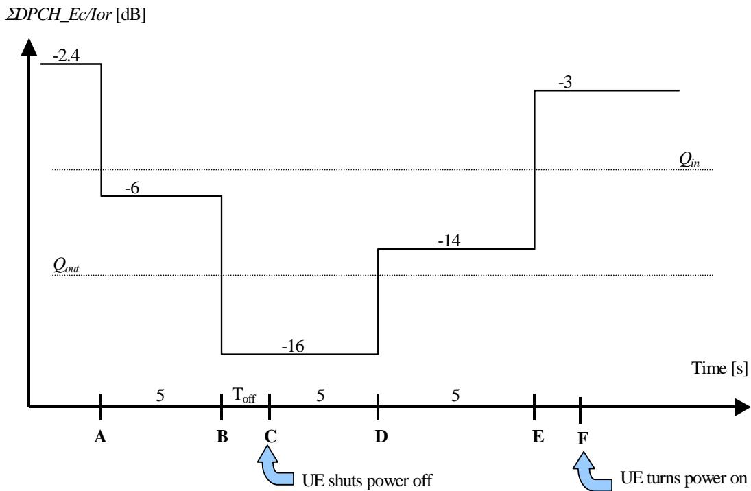
**Figure 5.4.5.2.2: Conditions for out-of-synch handling in the UE. The indicated thresholds  $Q_{out}$  and  $Q_{in}$  are only informative. Conditions apply for 1,28 Mcps TDD Option – continuous transmission**
