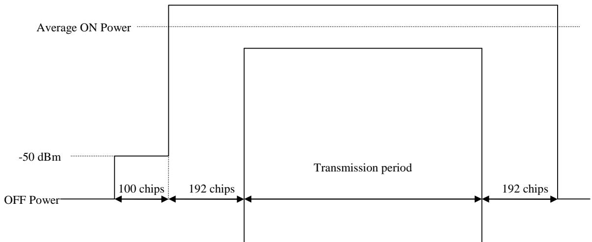
Figure 5.4.4.2.3: Transmit ON/OFF template for 7,68 Mcps TDD Option
