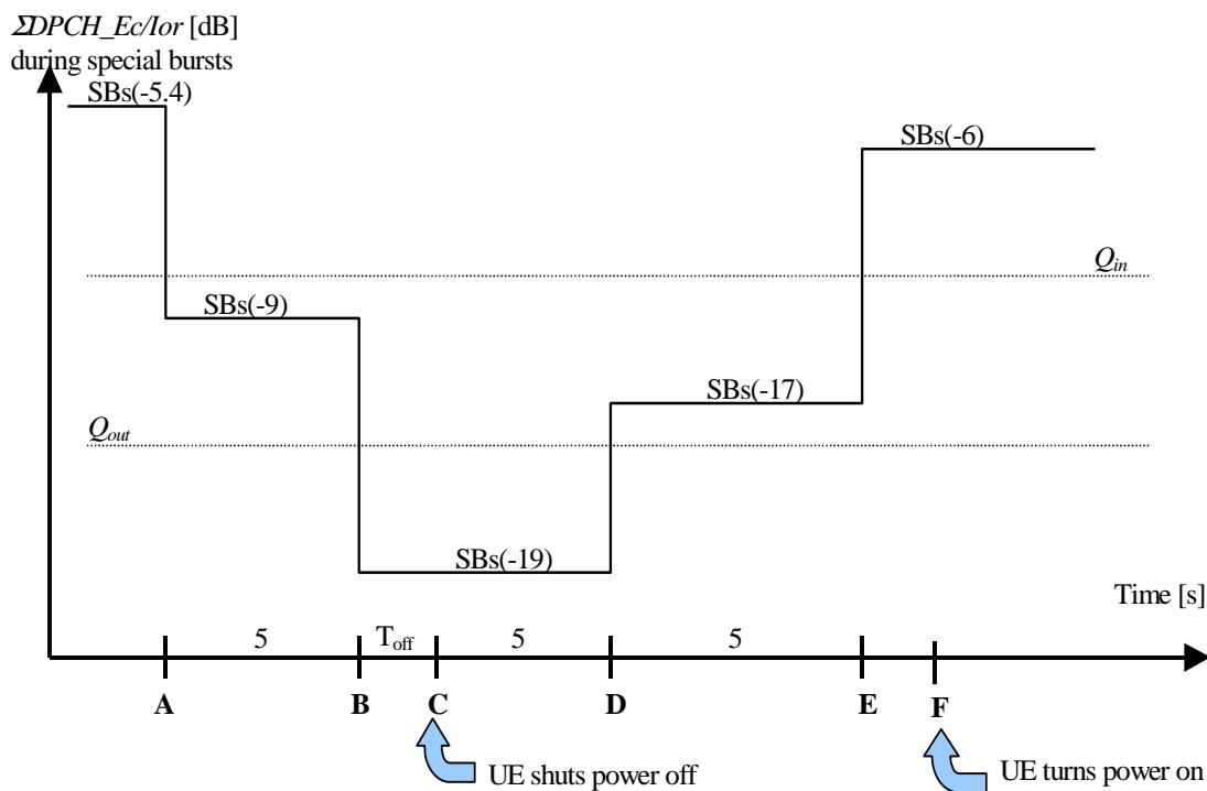
**Figure 5.4.6.2.2: Conditions for out-of-synch handling in the UE. The indicated thresholds  $Q_{out}$  and  $Q_{in}$  are only informative. Conditions apply for 1,28 Mcps TDD Option – discontinuous transmission**
