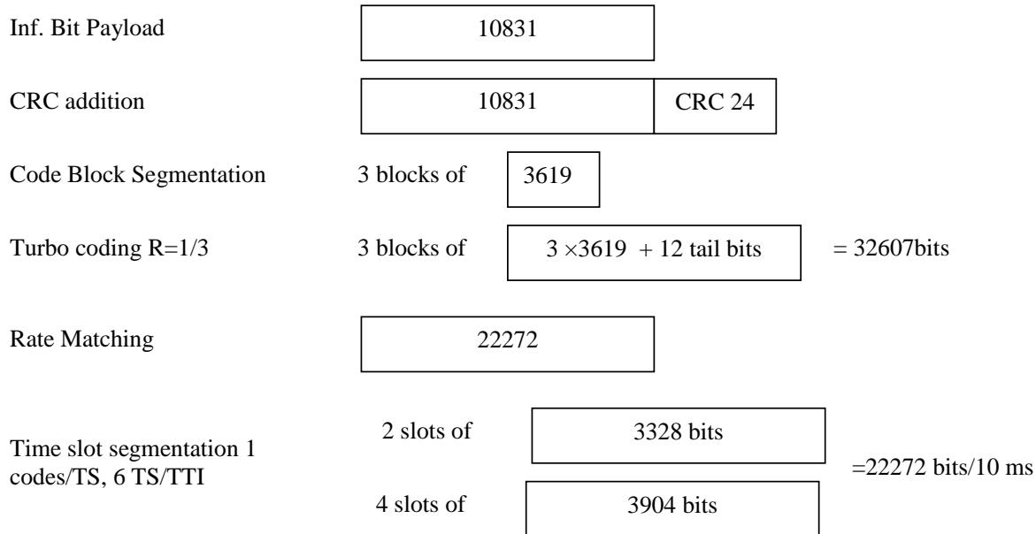
**Figure A.10: Coding for E-DCH FRC2 (3.84 Mcps TDD Option)****C.6.1.1.3 Fixed Reference Channel 3 (FRC3)****Table C.6.1.1c: E-DCH Fixed Reference Channel 3 (3.84 Mcps TDD Option)**
