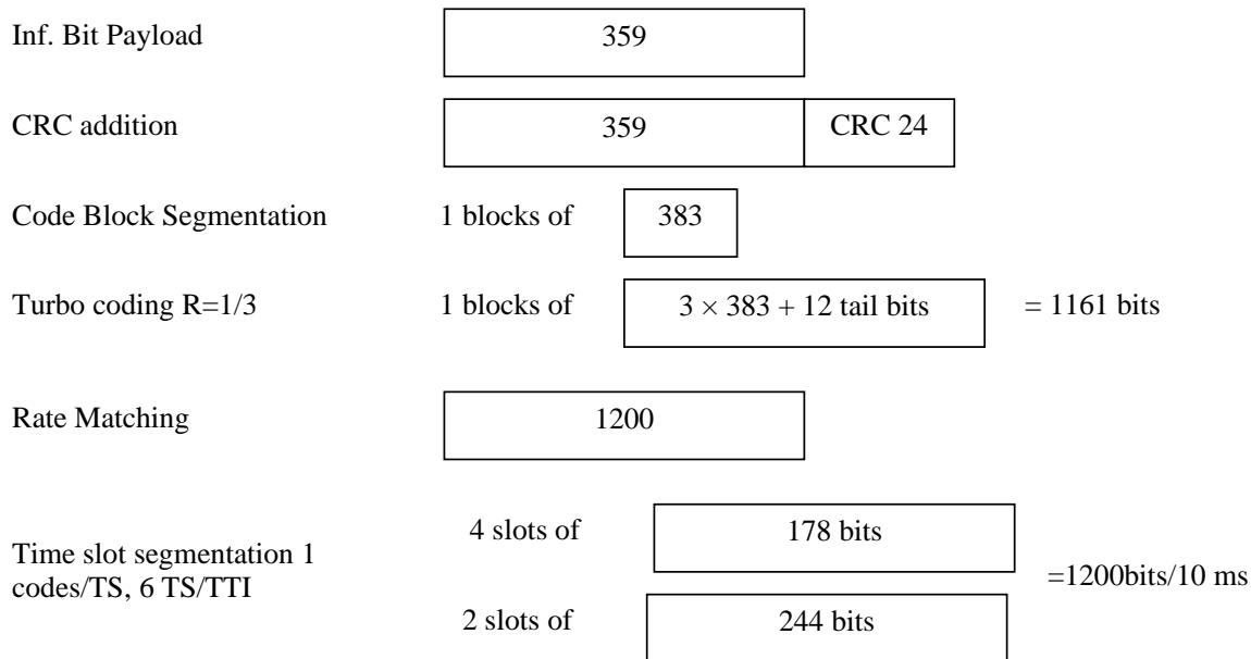
**Figure A.12: Coding for E-DCH FRC1 (7.68 Mcps TDD Option)****C.6.1.3.2 Fixed Reference Channel 2 (FRC2)****Table C.6.1.3b: E-DCH Fixed Reference Channel 2 (7.68 Mcps TDD Option)**
