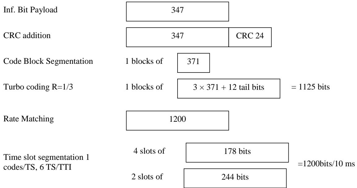
**Figure A.9: Coding for E-DCH FRC1 (3.84 Mcps TDD Option)****C.6.1.1.2 Fixed Reference Channel 2 (FRC2)****Table C.6.1.1b: E-DCH Fixed Reference Channel 2 (3.84 Mcps TDD Option)**
