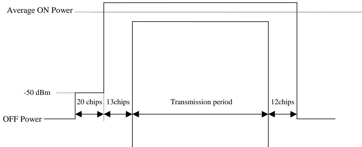
**Figure 5.4.4.2.2: Transmit ON/OFF template for 1,28Mcps TDD Option**
