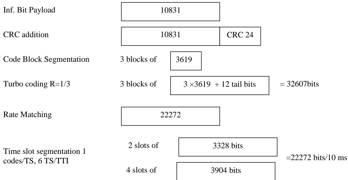
**Figure A.13: Coding for E-DCH FRC2 (7.68 Mcps TDD Option)****C.6.1.3.3 Fixed Reference Channel 3 (FRC3)****Table C.6.1.3c: E-DCH Fixed Reference Channel 3 (7.68 Mcps TDD Option)**
