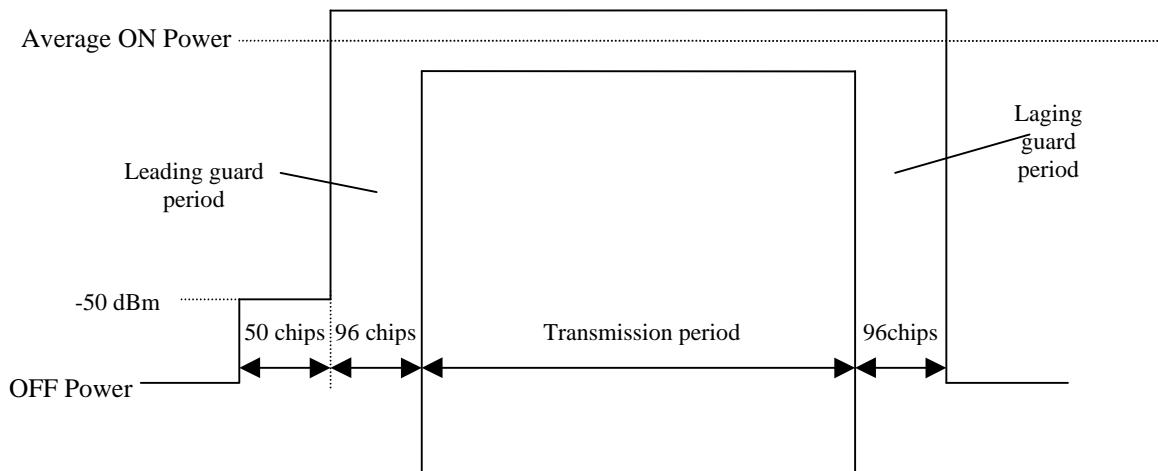
**Figure 5.4.4.2.1: Transmit ON/OFF template for 3,84 Mcps TDD Option**
