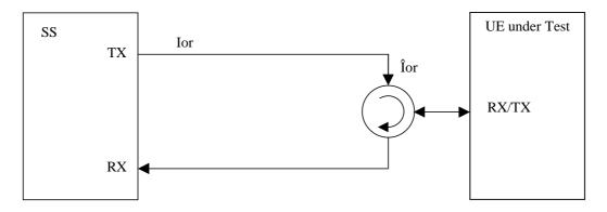
Figure A.3: Connection for Basic RX Test
