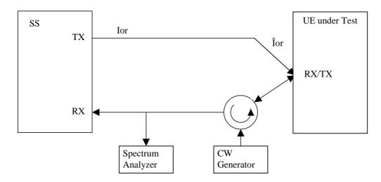
Figure A.2: Connection for TX Intermodulation Test
