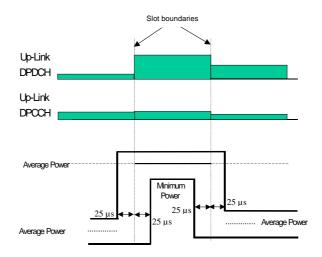
Figure 5.6.1: Transmit template during TFC change
