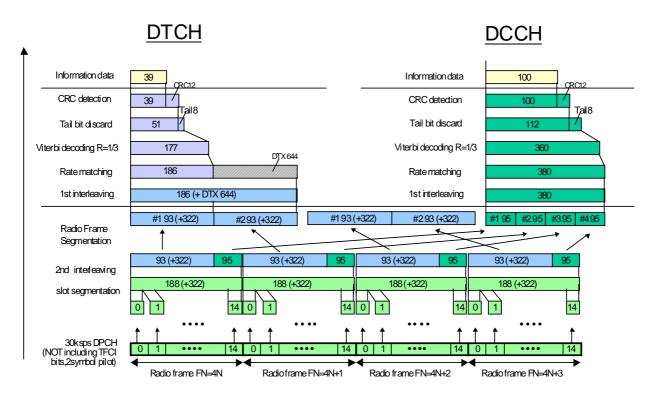
Figure C.4.3 (informative): Channel coding of DL reference measurement channel for BTFD (Rate 3)
