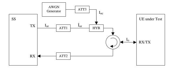
Figure A.9: Connection for Static Propagation Test
