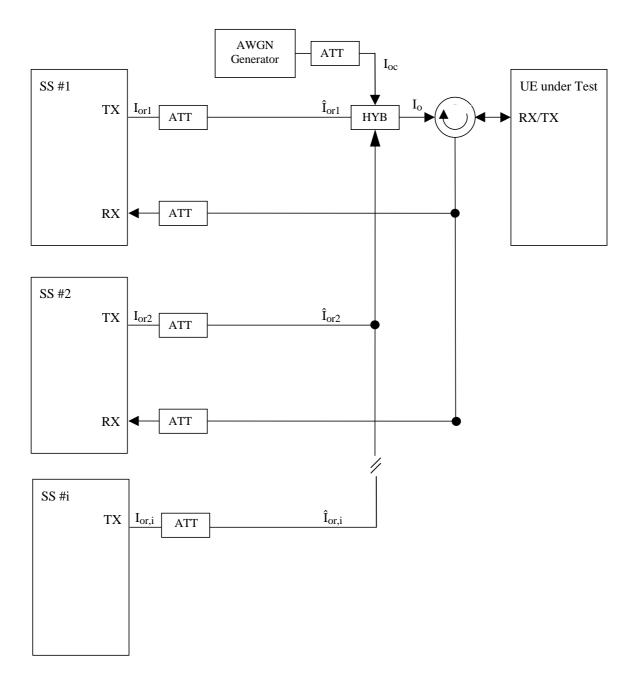
Figure A.14: Connection for cell reselection single carrier multi cell
