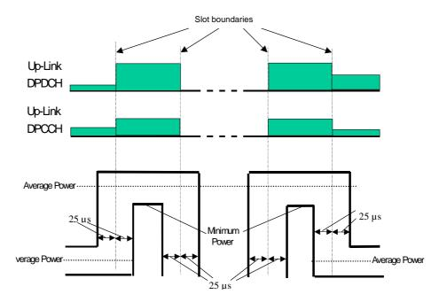
Figure 5.7.1: Transmit template during Compressed mode
