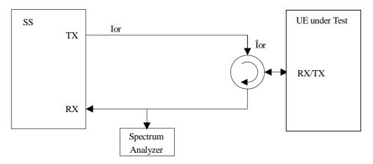
Figure A.8: Connection for Spurious Emission Test
