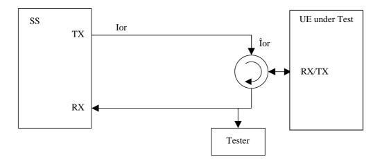
Figure A.1: Connection for Basic TX Test
