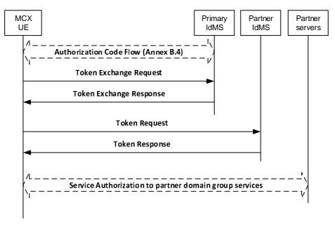
Figure 5.1.4.2-2: Token exchange procedure
