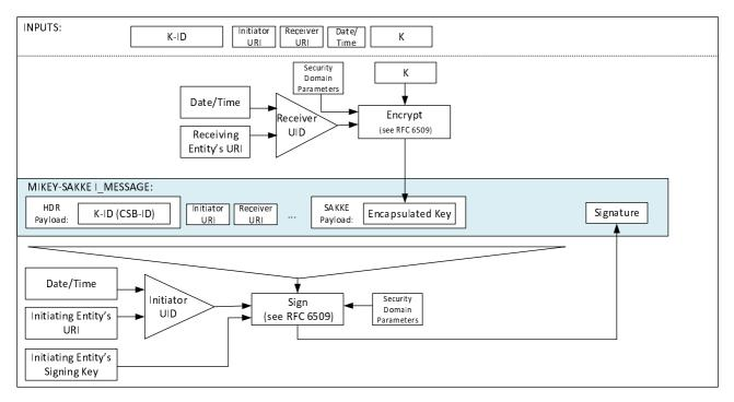
Figure 5.2.2-1: Common key distribution mechanism
