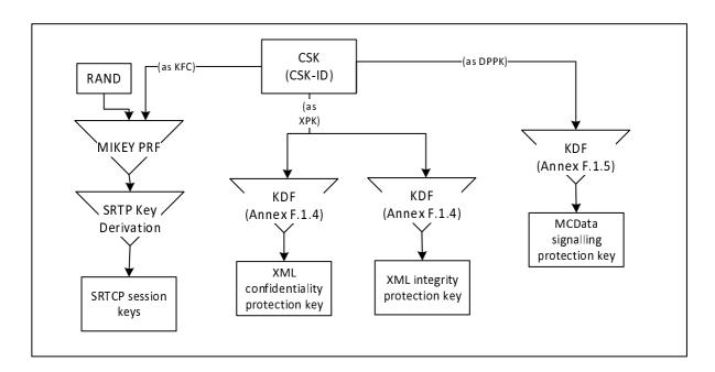
Figure 9.2.1-1: Uses of the Client-Server Key
