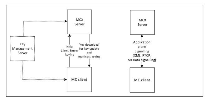
Figure 4.3.4-1: Application plane signalling security
