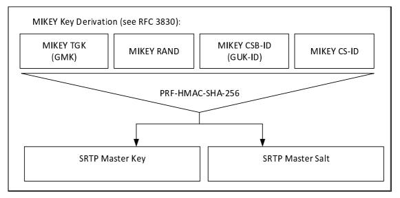
Figure 7.4.2-1: Key Derivation for media stream protection
