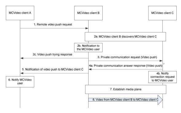
Figure 7.2.8.3-2: Off-network remotely initiated video push
