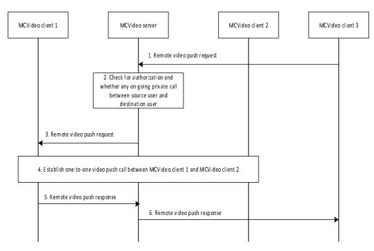
Figure 7.2.8.3-1: On-network remotely initiated video push
