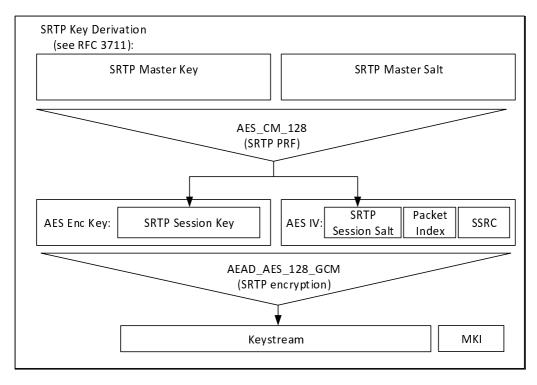
Figure 7.5.1-1: Security mechanism for media stream protection
