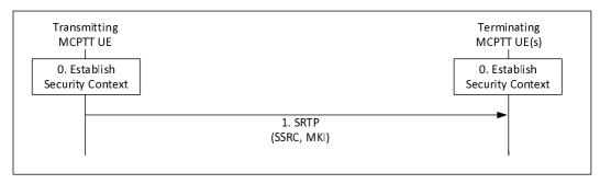
Figure 7.5.2-1: Security procedure for media stream protection
