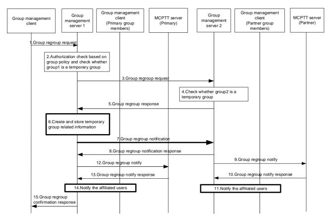
Figure 7.3.3.3-1: Group regroup security procedure (multiple MC domains)
