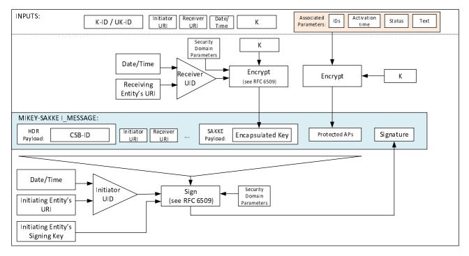
Figure 5.2.4-1: Common key distribution mechanism with associated parameters
