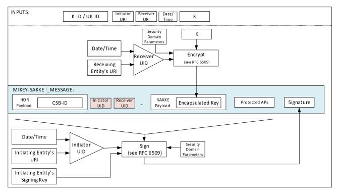
Figure 5.2.6-1: Common key distribution mechanism with identity hiding
