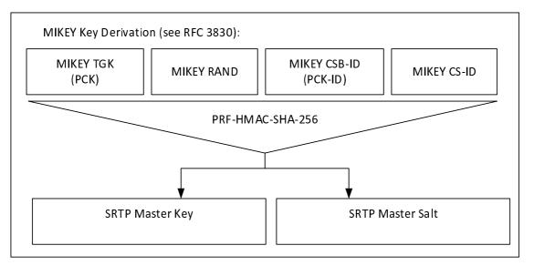
Figure 7.4.1-1: Key Derivation for media stream protection
