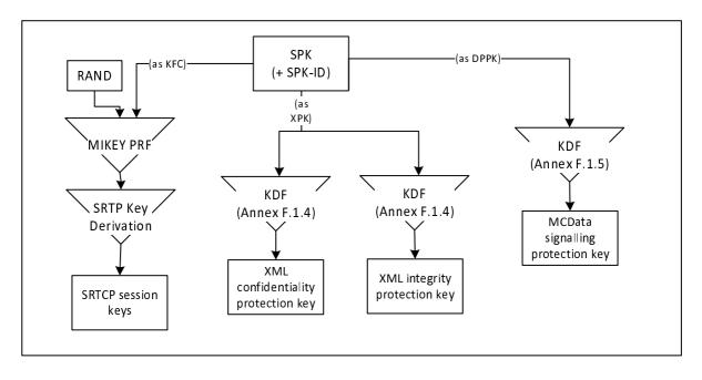
Figure 9.2.3-1: Uses of the Signalling Protection Key
