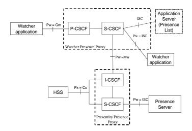
Figure 1: The Location of the Presence Server and the Presence List Server from an IMS point of view
