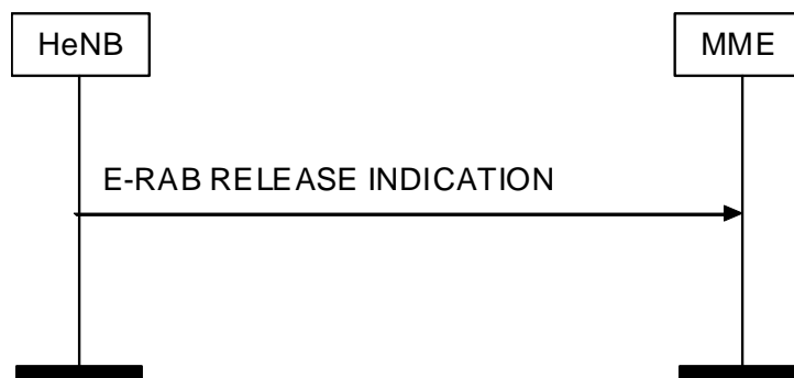
Figure 9 E-RAB Release INDICATION procedure. Successful operation
