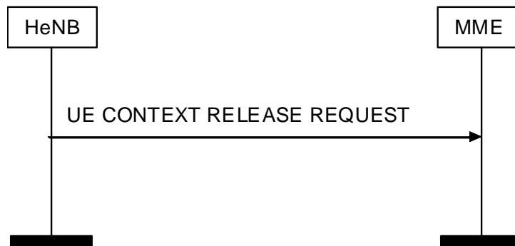
Figure 7 UE Context Release Request procedure. Successful operation
