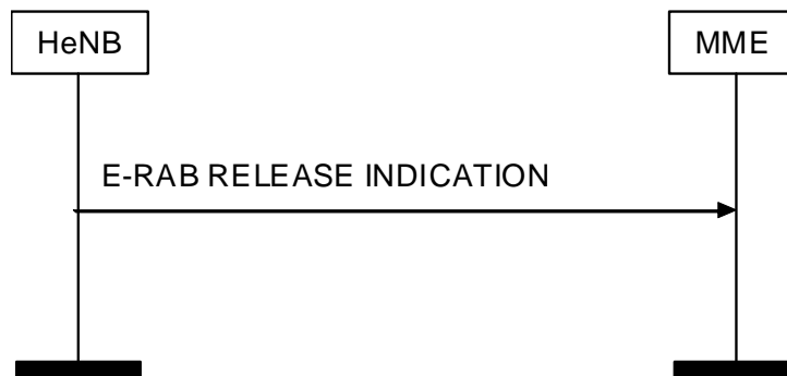
Figure 9 E-RAB Release INDICATION procedure. Successful operation
