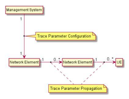
Figure 4.3.2 : Architecture for Signalling Based Activation/Deactivation required for Service Level Tracing for IMS at the IMS NE
