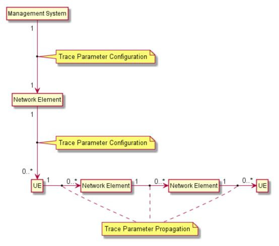
Figure 4.3.1: Architecture for Signalling Based Activation/Deactivation required for Service Level
