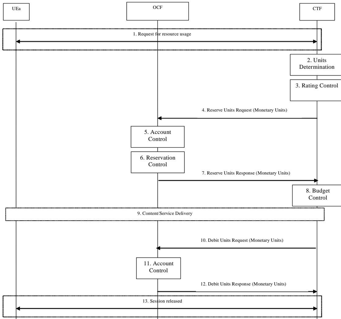
Figure 5.2.2.2.3.1: ECUR - Centralized Unit Determination and Centralized Rating
