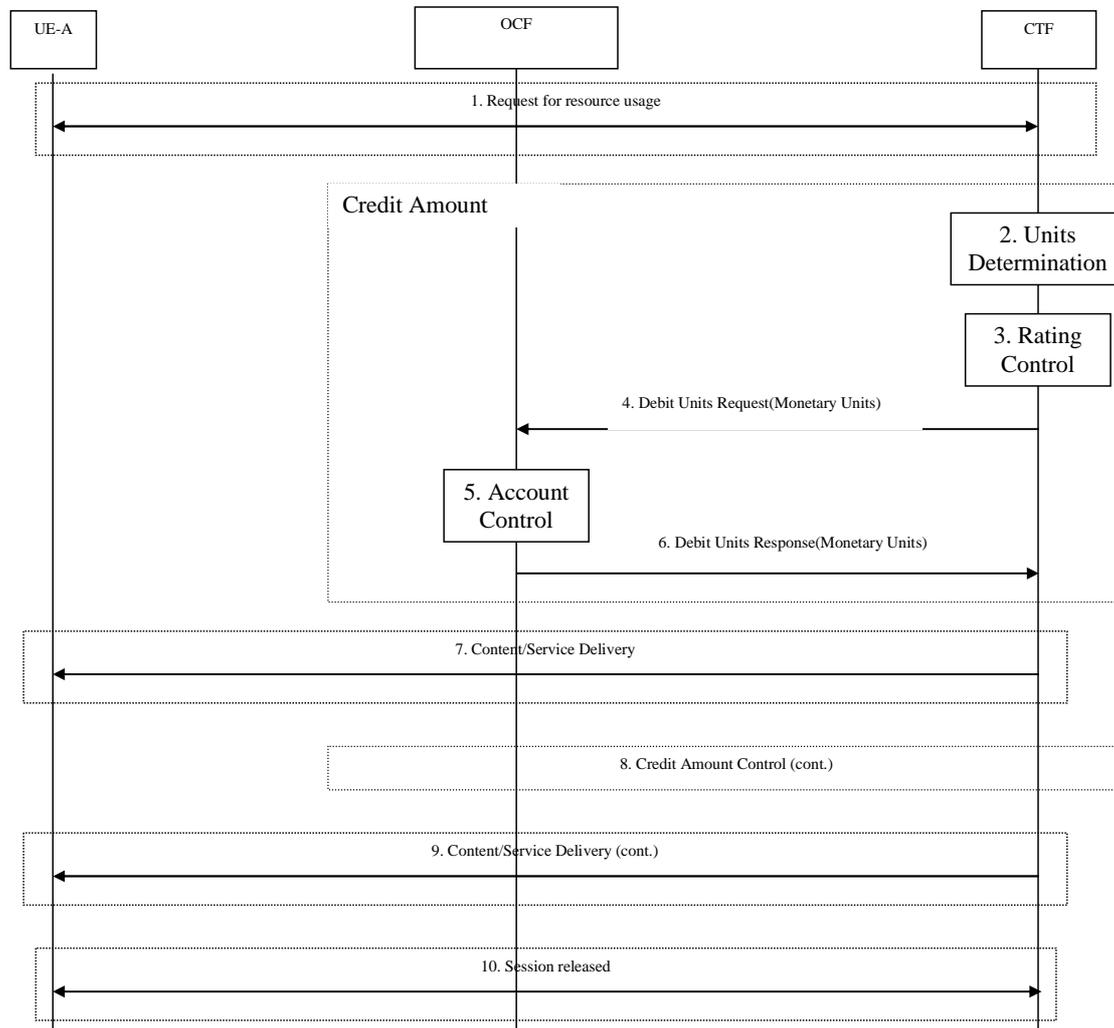
**Figure 5.2.2.1.3.1: IEC - Decentralized Rating and Decentralized Unit Determination**
