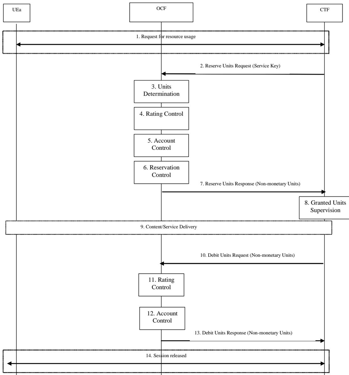
Figure 5.2.2.2.1: ECUR - Centralized Unit Determination and Centralized Rating
