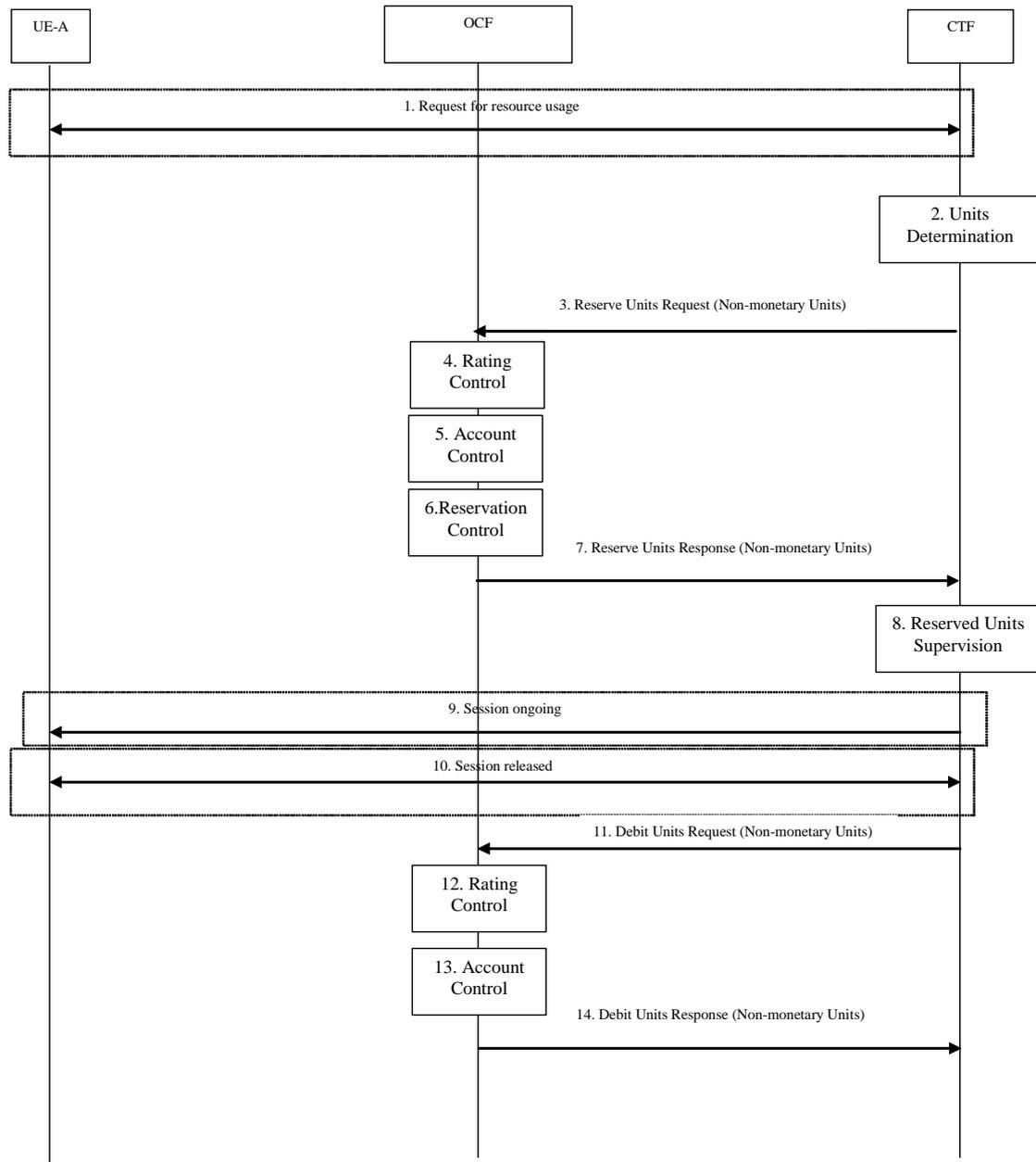
**Figure 5.2.2.3.1.1: SCUR - Decentralized Unit Determination and Centralized Rating**
