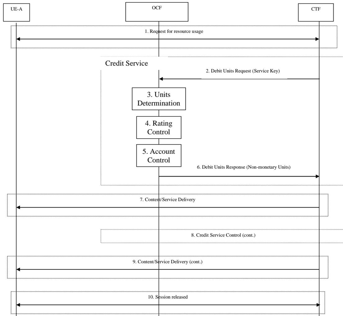
**Figure 5.2.2.1.2.1: IEC - Centralized Rating and Centralized Unit Determination**
