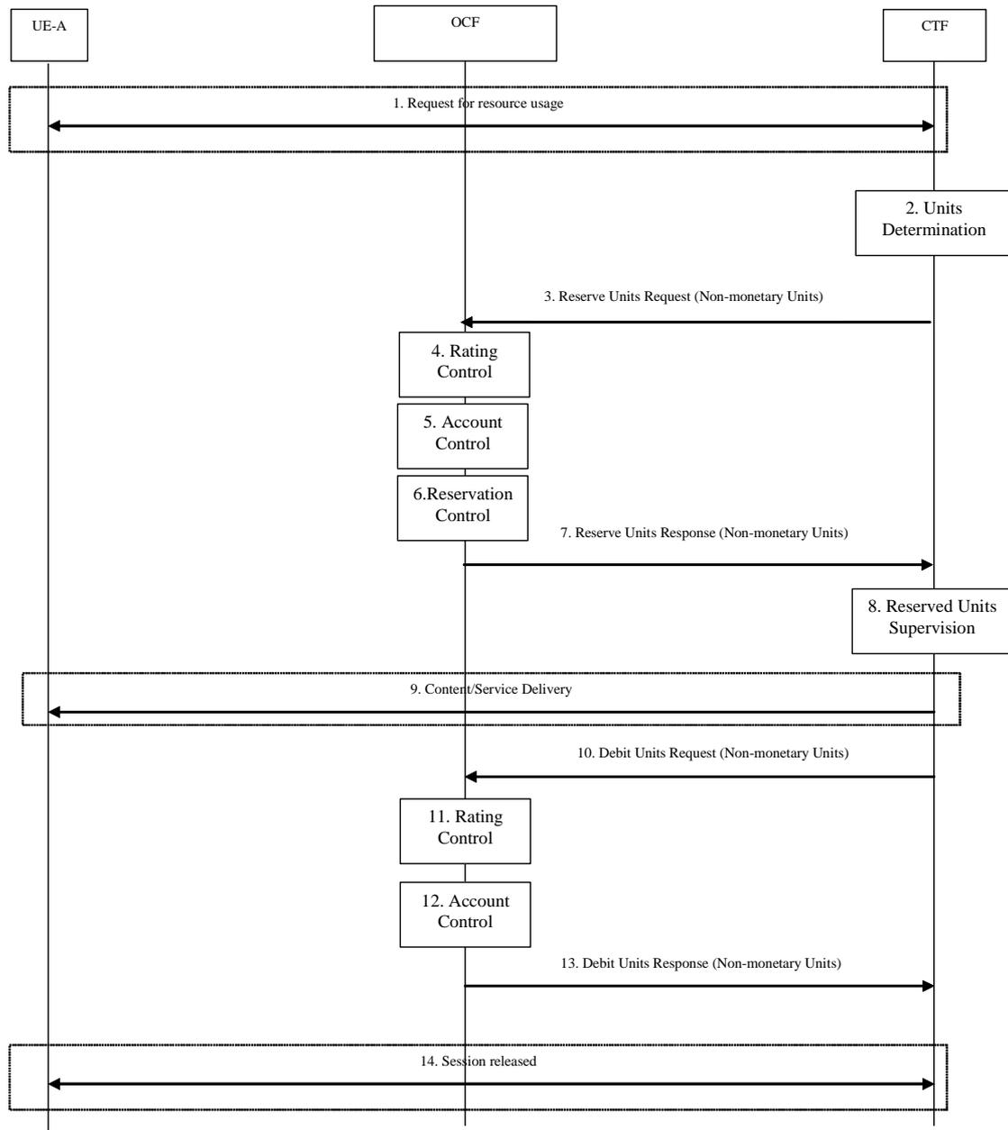
**Figure 5.2.2.2.1.1: ECUR - Decentralized Unit Determination and Centralized Rating**
