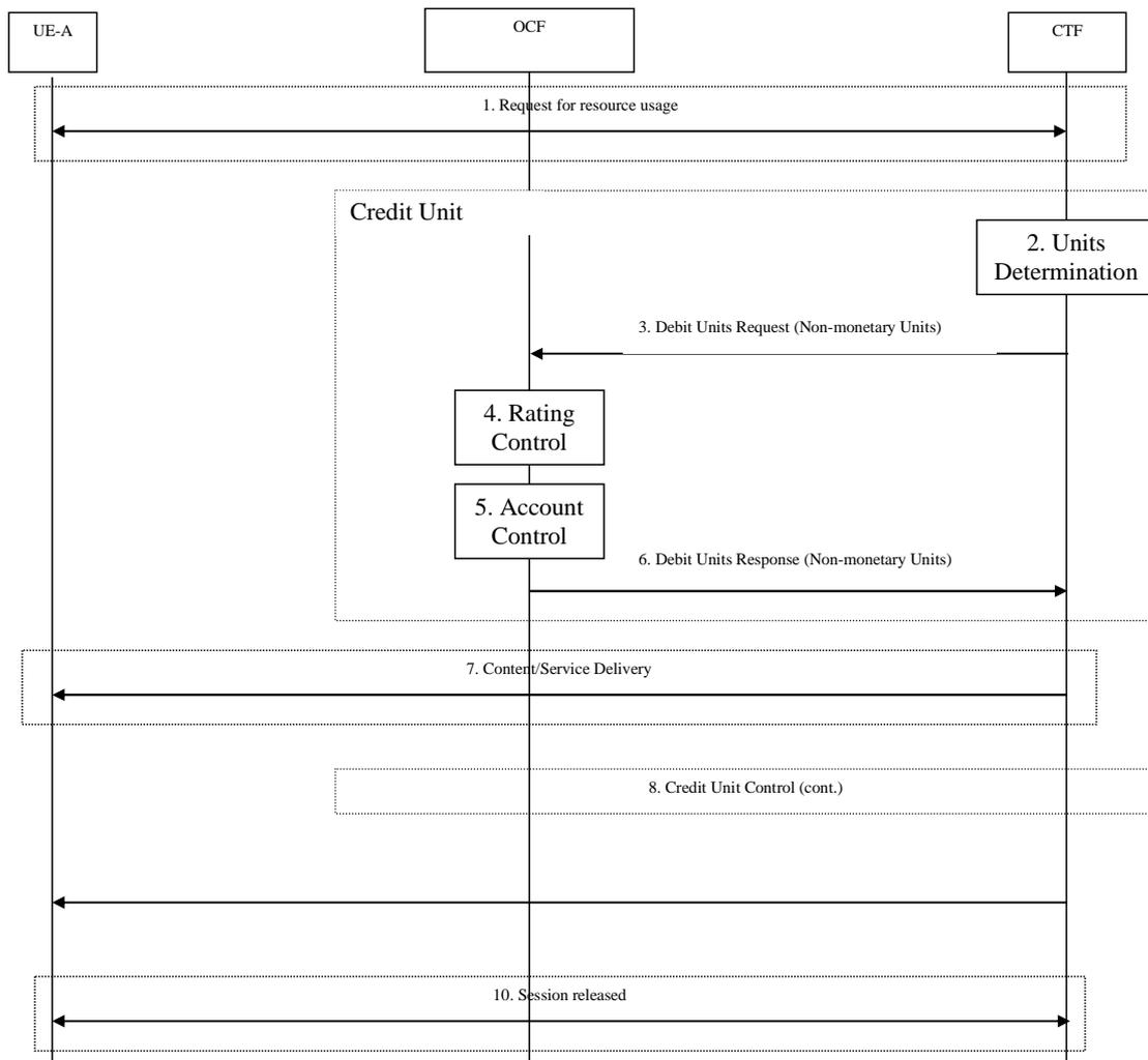
**Figure 5.2.2.1.1.1: IEC - Centralized Rating and Decentralized Unit Determination**
