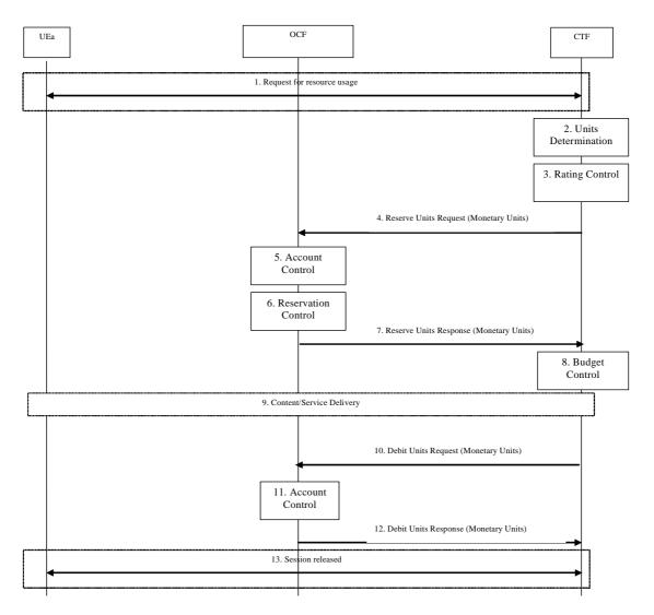
Figure 5.2.2.3: Event Charging with Reservation / Centralized Unit Determination and Centralized Rating
