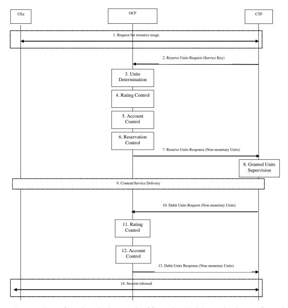
Figure 5.2.2.2: Event Charging with Reservation / Centralized Unit Determination and Centralized Rating
