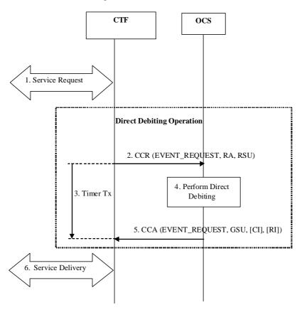
Figure 6.3.3: IEC Direct Debiting Operation
