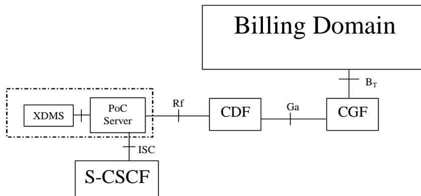
**Figure 4.2: Charging architecture for PoC offline charging**
