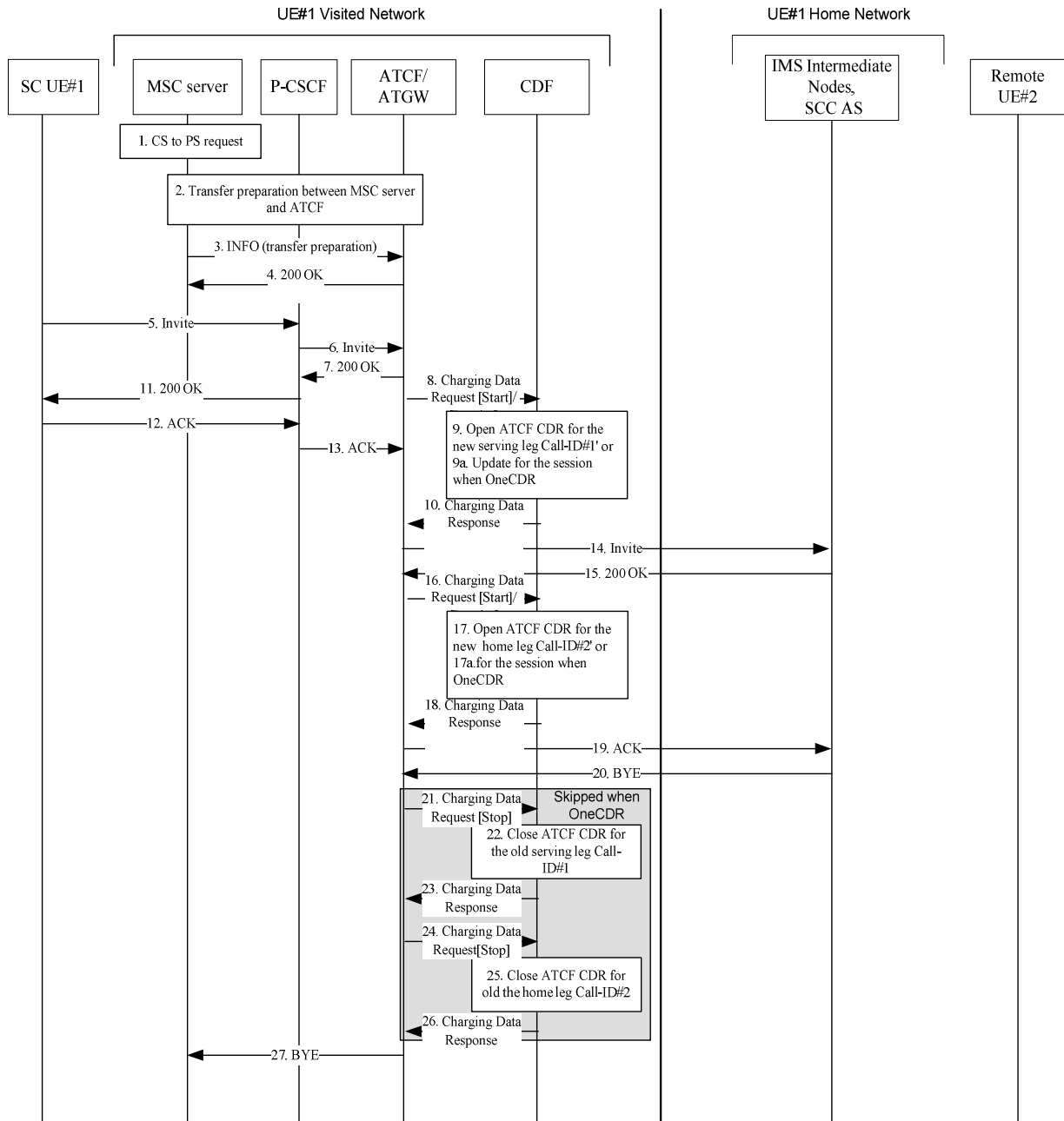
Figure 5.2.2.1.22.4.1: Message sequence chart UE session transfer CS to PS using ATCF
