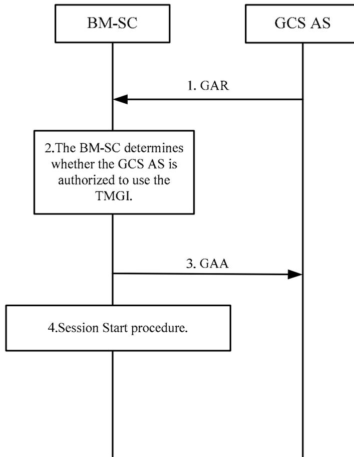
**Figure A.2.1.1: Activate MBMS bearer Procedure**
