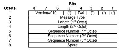
NOTE 0: (\*) This bit is a spare bit. It shall be sent as '0'. The receiver shall not evaluate this bit.
