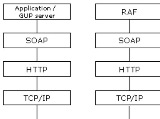
**Figure 7.7.2** GUP Rp reference point protocol architecture
