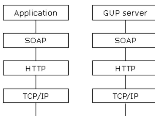
**Figure 7.2.1** GUP Rg reference point protocol architecture
